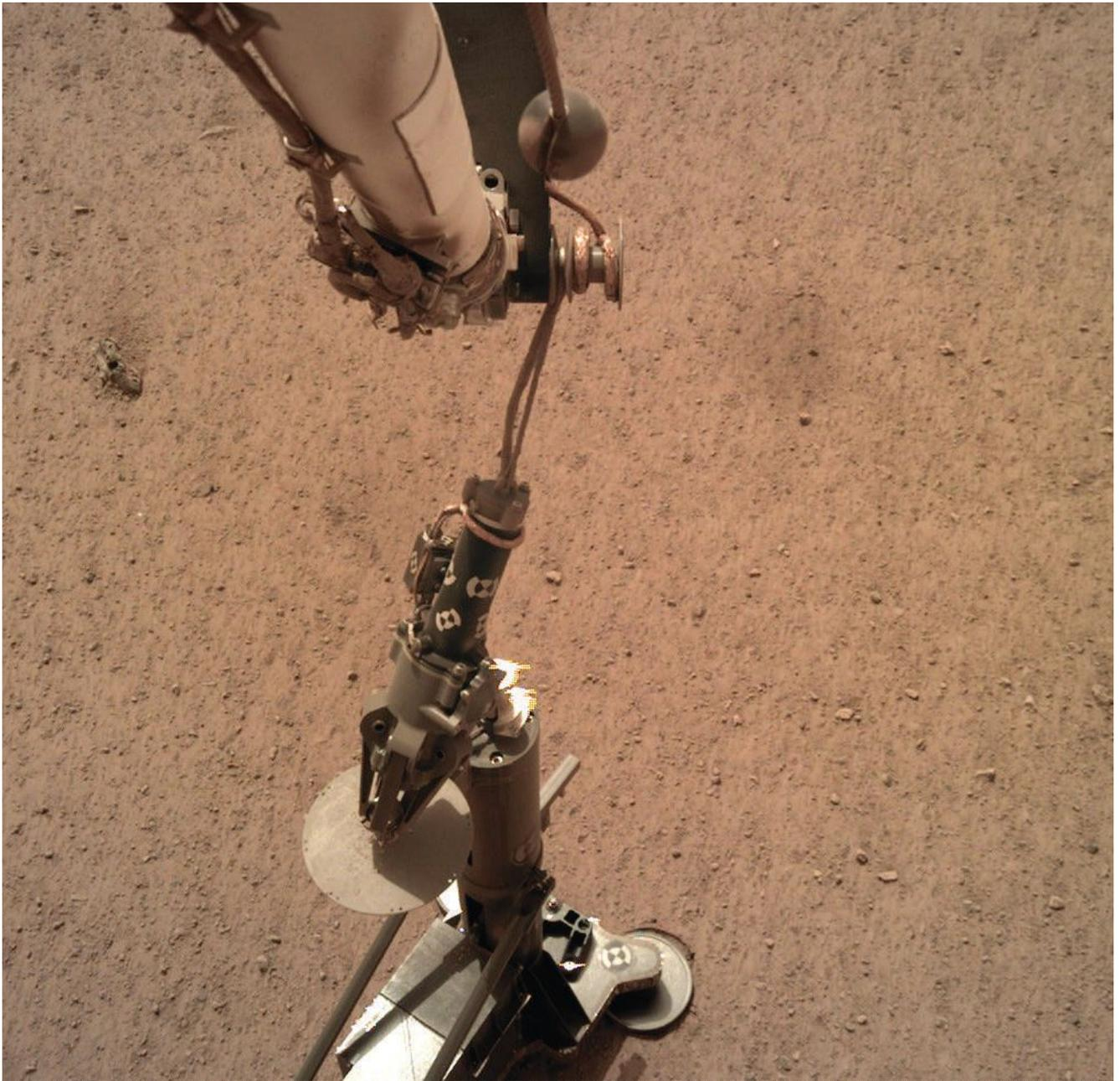
Prior to the Mole's deployment, Banerdt told me he thought the Mole had a 75 percent to 80 percent chance of reaching 5 meters. That probability came close to a prior estimate, which assumed the Mole could get past rocks up to 15 centimeters in diameter or those oriented with their surfaces at a 45-degree angle to the Mole's path.
