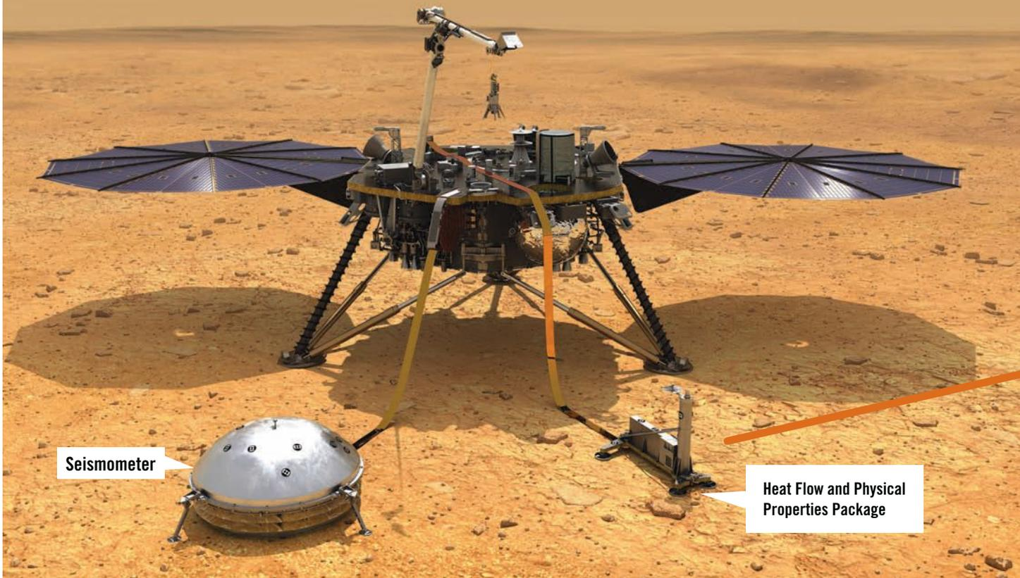
sponsibly, partly to try to keep planets as pristine as possible for more study. The Mole is designed to dig only as deeply as it needs to — 3 meters to 5 meters, according to scientists, to get good data.
