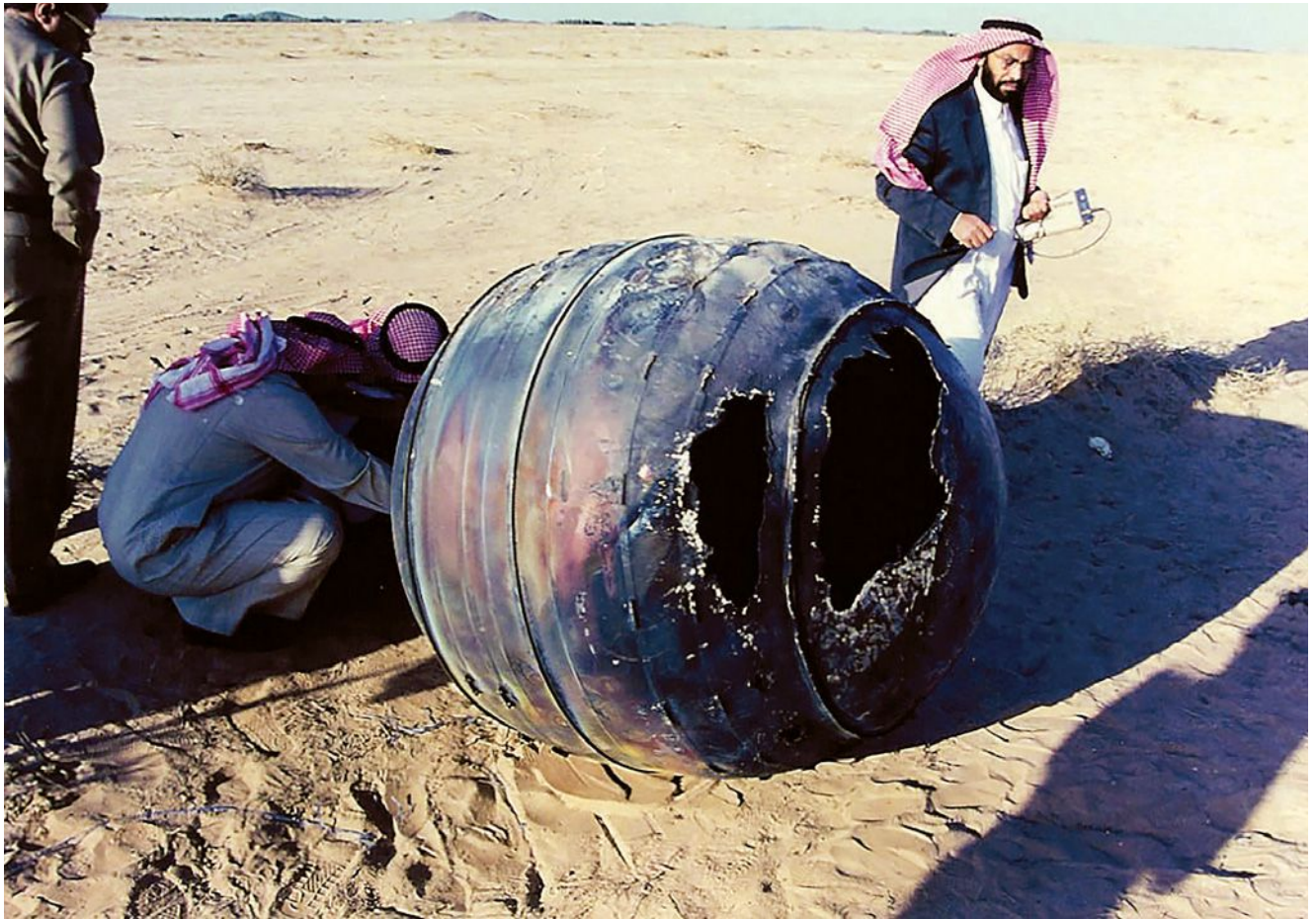
▲ A Delta II third stage reentered the atmosphere in 2001. Its titanium motor casing landed in Saudi Arabia. NASA
