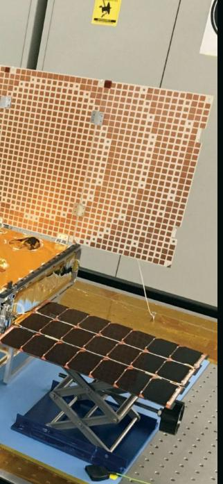
NASA's Mars Cube One spacecraft are one example of how Mars could be explored via less expensive means. The pair of cubesats, pictured here in 2018 at NASA's Jet Propulsion Lab in California, relayed X-band signals from NASA's InSight lander, providing mission controllers real-time status updates about the InSight lander's November 2018 entry, descent and landing on Mars.
