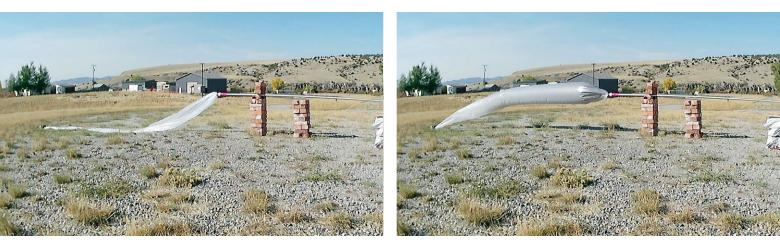
from granules of a metal hydride in the drum to form hydrogen gas. The whoosh was the sound of gas slowly inflating the plastic bag, a successful result that was met with a subdued reaction from the NASA managers in the group.
