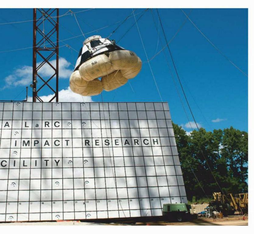
Instead of the Soyuz's heavy retrothrusters, Boeing designed six lightweight airbags for the Starliner (being tested at Langley Research Center, left) that should put a somewhat more comfortable bounce in its drop back to Earth.
