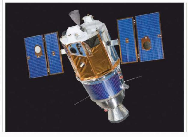
Above: Lidar measurements of lunar topography from the Clementine mission. Left: The Clementine model; its interstage and solid rocket motor (bottom half) were discarded before insertion into lunar orbit.
