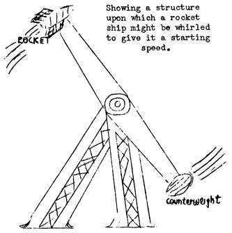
We now come to an entirely different idea. Take advantage of centrifugal force, which tends to throw off an object in a direction tangential to the circle and at the same speed. This tendency is precise. The suggestion has been made by M. Esnault-Pelterrie to suspend a space-ship after the fashion of a car in a huge Ferris wheel. This wheel will whirl around at increasing speed and finally the car is released and flies off into space.
