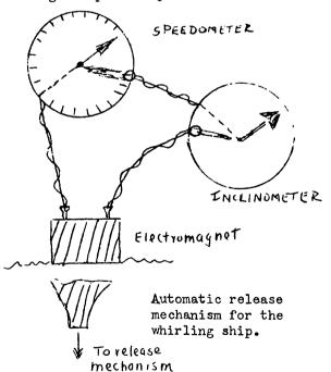
If the release of the ship from the wheel be by manual control, he must push the button at the exact moment, setting up an electric connection which will operate the release and permit the ship to fly off on its course and at the same time start the rocket motors.
