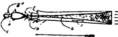
FIG. 19. Melot nozzle drive, experimental arrangement A = combustion air admission B = spark plugs for starting Br. = burners C = fuel admission D = nozzles G = gas jet I = mixture air T = combustion chamber mouth
