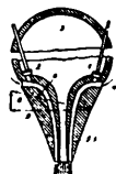
Fig. 54. S. H. Akimoff, 1934. Additional air over aerofoil profiles: sucking away of boundary layer
