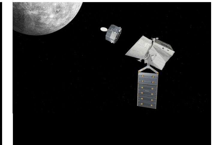
SEPARATION OF MERCURY MAGNETOSPHERIC ORBITER
