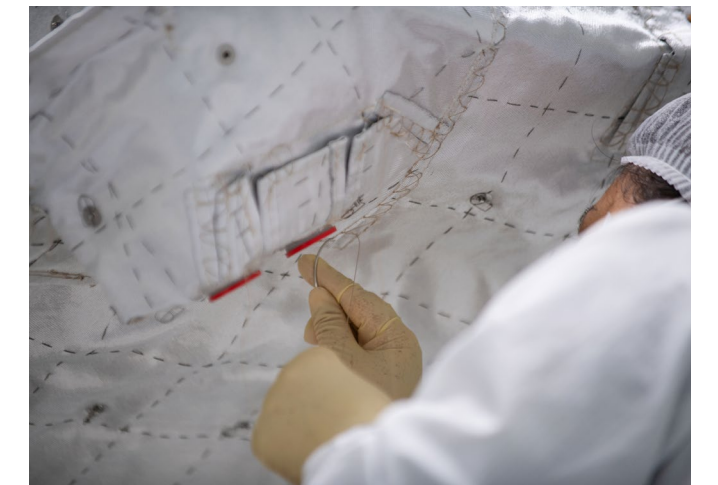
HAND-SEWN INSULATION BLANKETS
