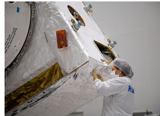
SEWING MTM INSULATION BLANKETS
