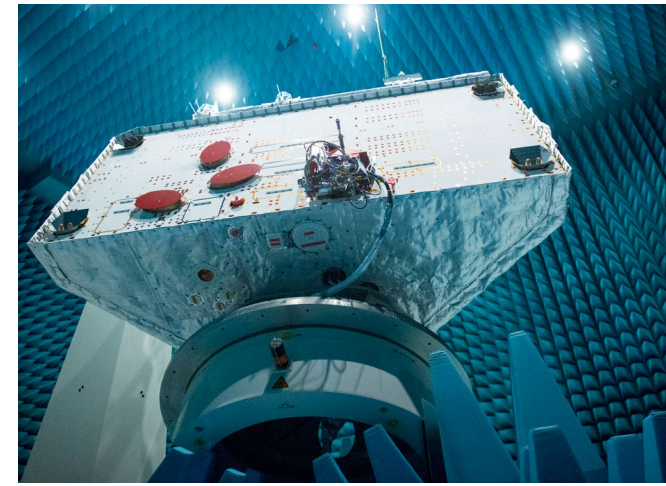
RADIO TESTING OF BEPICOLOMBO ORBITER
