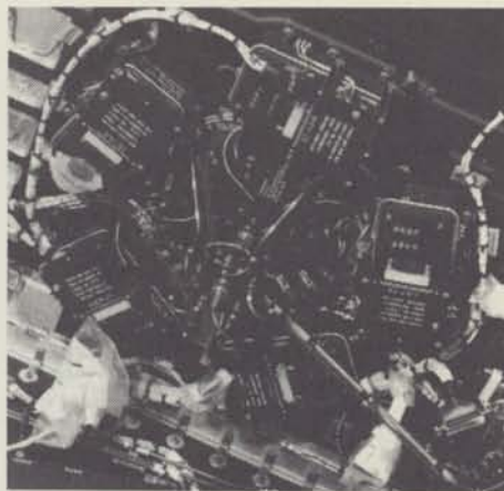
Marecs spacecraft transistor power amplifier for L-band transmissions to maritime traffic.
