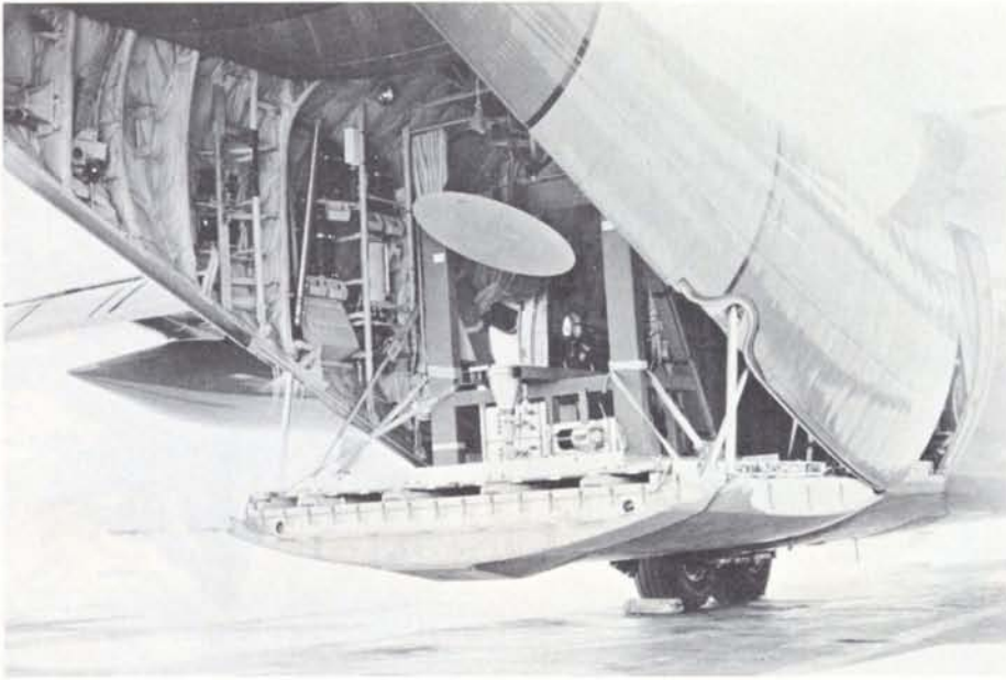
Figure 4 — The three-frequency radiometer system mounted on the open ramp of the C-130 aircraft with a scanning offset parabolic antenna. The aircraft is flown with the ramp open during measurements, with the antenna beams directed at 50^\circ to the ground in a 1 Hz conical scan.
