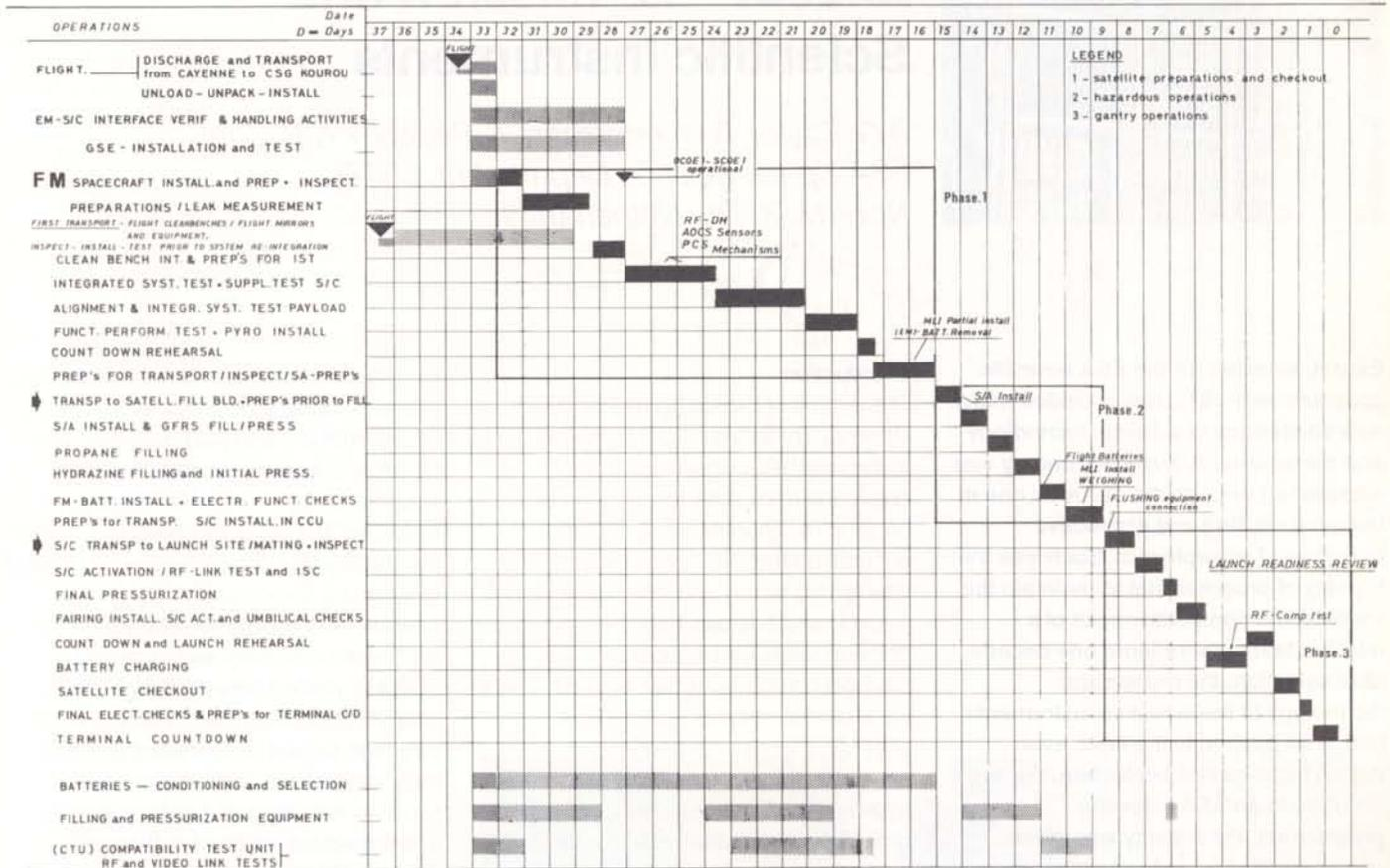
pyrotechnics circuitry and adjustments to mechanisms/appendages, partial installation of superinsulation, and installation of pyrotechnics will take place during this phase, for reasons of internal accessibility and prerequisite to the hazardous operations in Phase 2.
