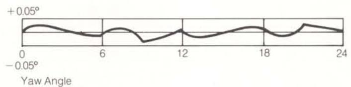
1982, when the attitude was controlled by four duty cycles of the south array per day. In comparison with Figure 8, it can be seen that: (a) the roll angle remains comfortably within the thresholds of plus and minus  $0.05^\circ$ , and (b) yaw performance is systematically as good as roll performance.
