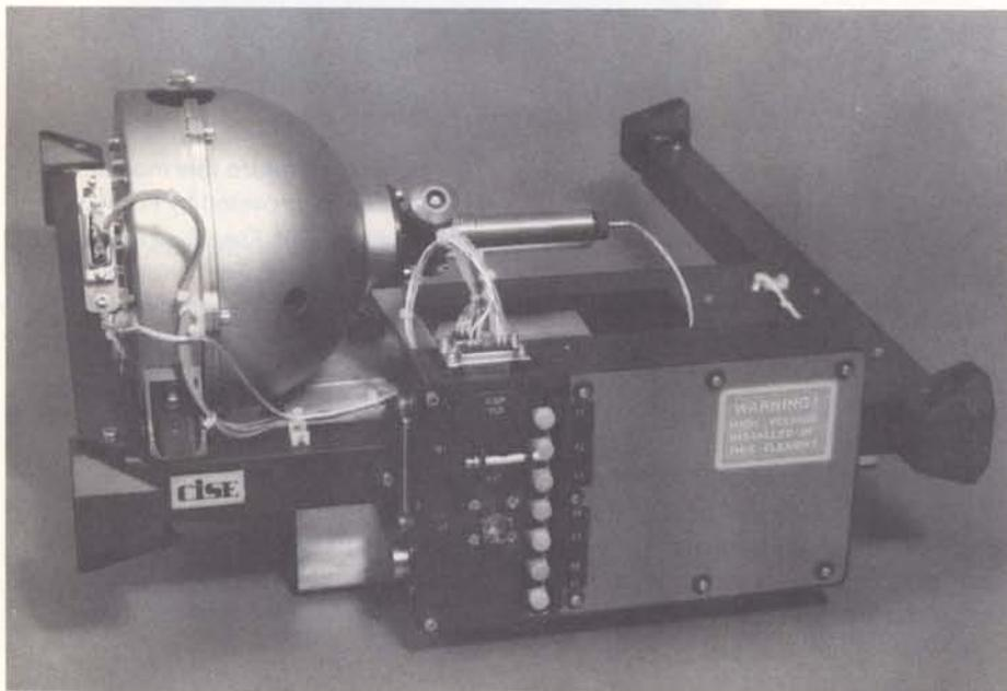
Figure 8 – The reactor chamber for the crystal-growth from solution experiments (ES 332/333)
