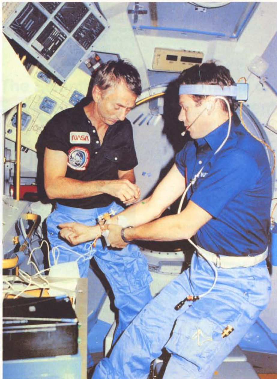
Figure 3 — Crew members Robert Parker and Ulf Merbold carrying out a 'ballistocardiography' investigation in which the recoil acceleration resulting from bodily blood motion is measured with the help of supersensitive accelerometers.
