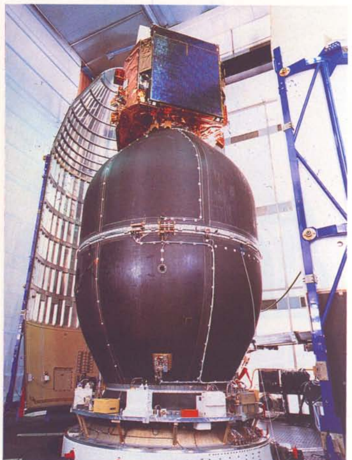
Mating of the SYLDA and Ariane-3 third stage
