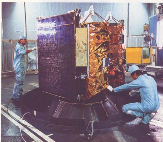
Mating of the SYLDA and Ariane-3 third stage
