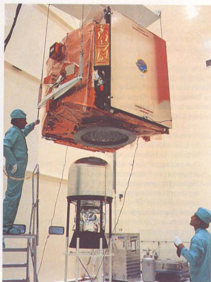
Mating of ECS-2 and apogee boost motor
