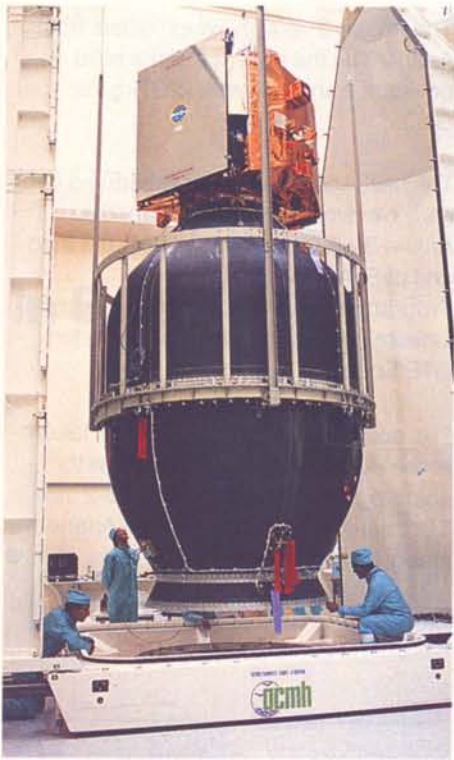
Transportation of the SYLDA to the launch tower
