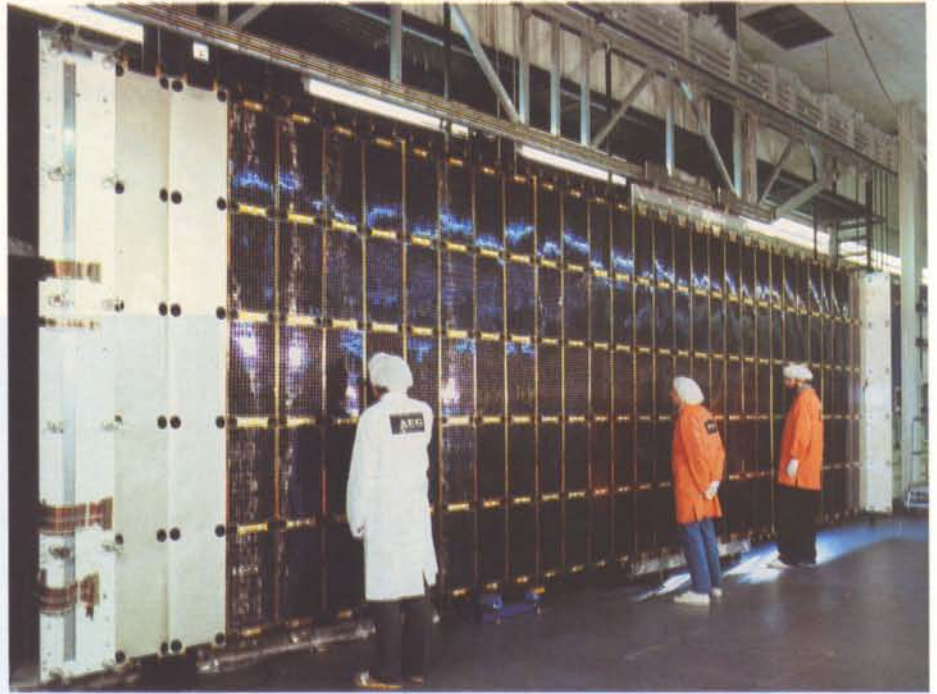
Figure 7 — Solar-array flight blankets for: (a) Olympus (formerly L-Sat); (b) Space Telescope
