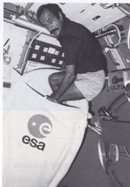
Wubbo Ockels entering the ESA sleep restraint system (currently under patent application), which provides an even distribution of pressure over the astronaut's body by means of inflatable tubes.
