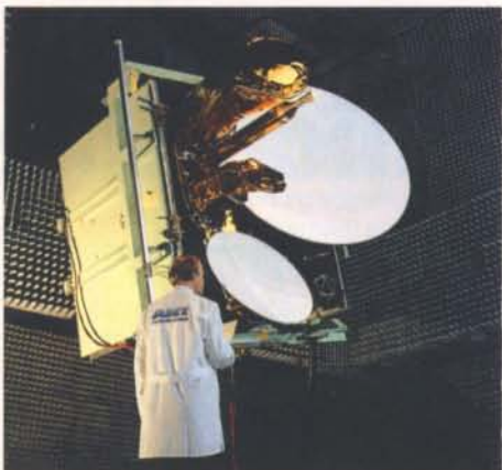
The German Telecommunications Satellite DFS Kopernikus: Payload system under orbital test conditions.
