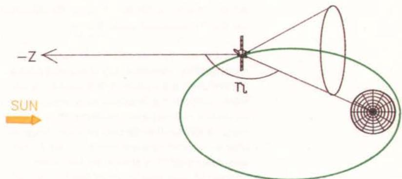
Figure 3. Earth acquisition in transfer orbit
