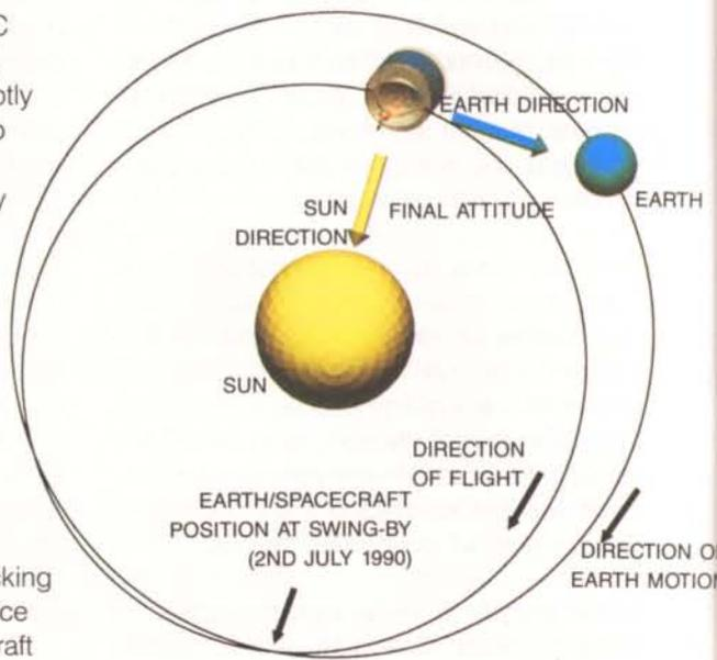
**Figure 7.** Orbital and attitude geometry after reactivation
