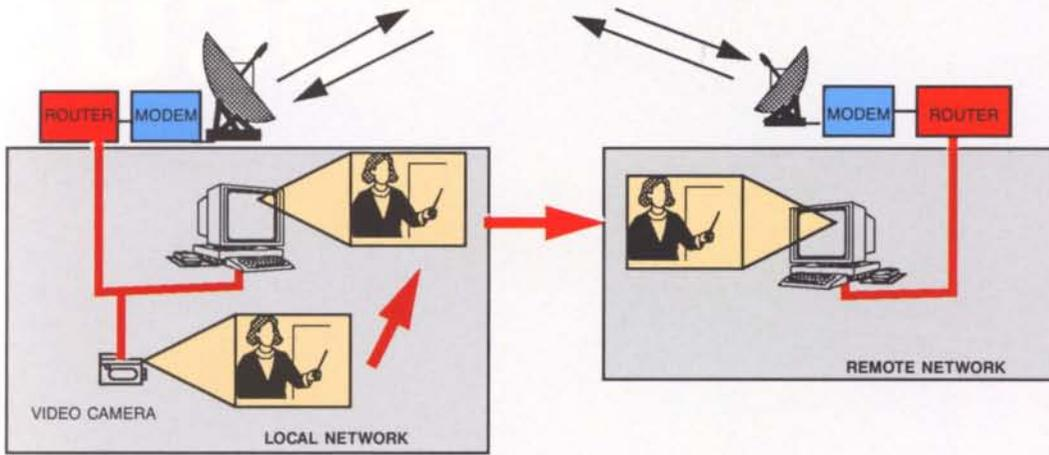
Figure 4. The setup for the video-frame transmission test
