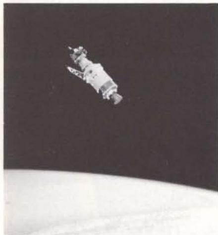
Cover: The Ulysses payload assembly (spacecraft + IUS + PAM-S) after deployment from Space Shuttle 'Discovery' (see page 109)
