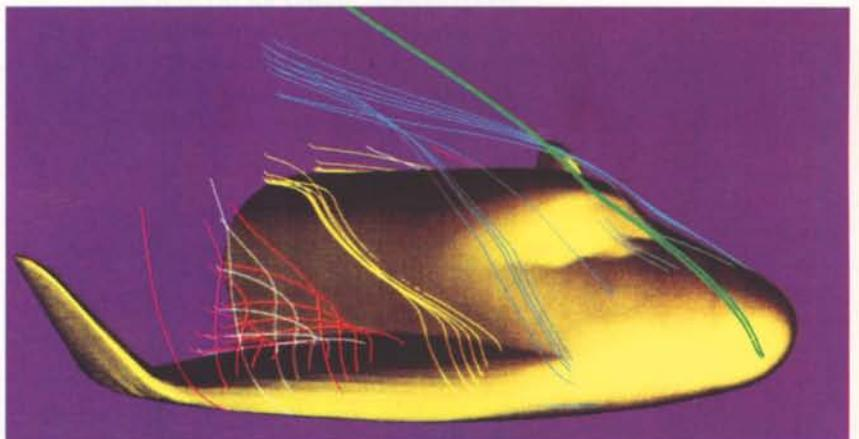
Figure 15. An example of particle-tracing (flow streamlines) around the Hermes vehicle
