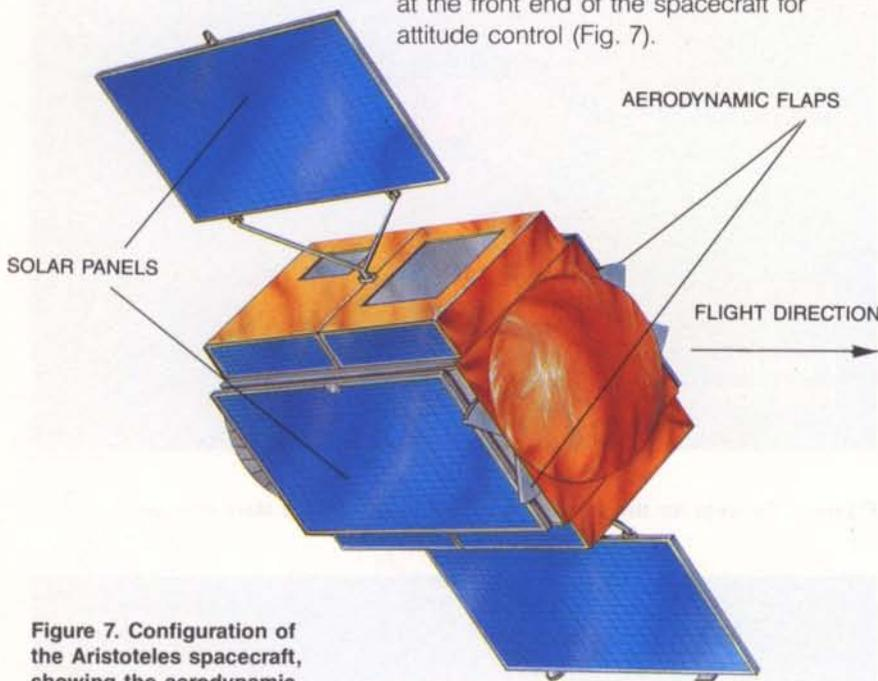
Figure 7. Configuration of the Aristoteles spacecraft, showing the aerodynamic flaps for attitude control
