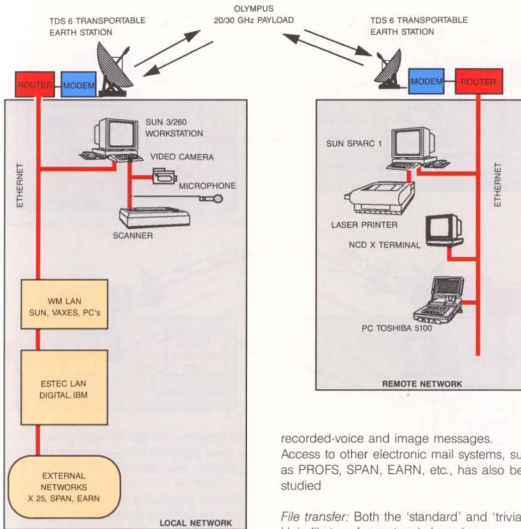
Figure 1. Hardware configuration for the computer-networking experiment
