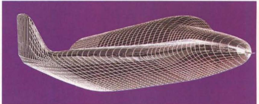
Figure 13. A typical surface grid for the Hermes spaceplane
