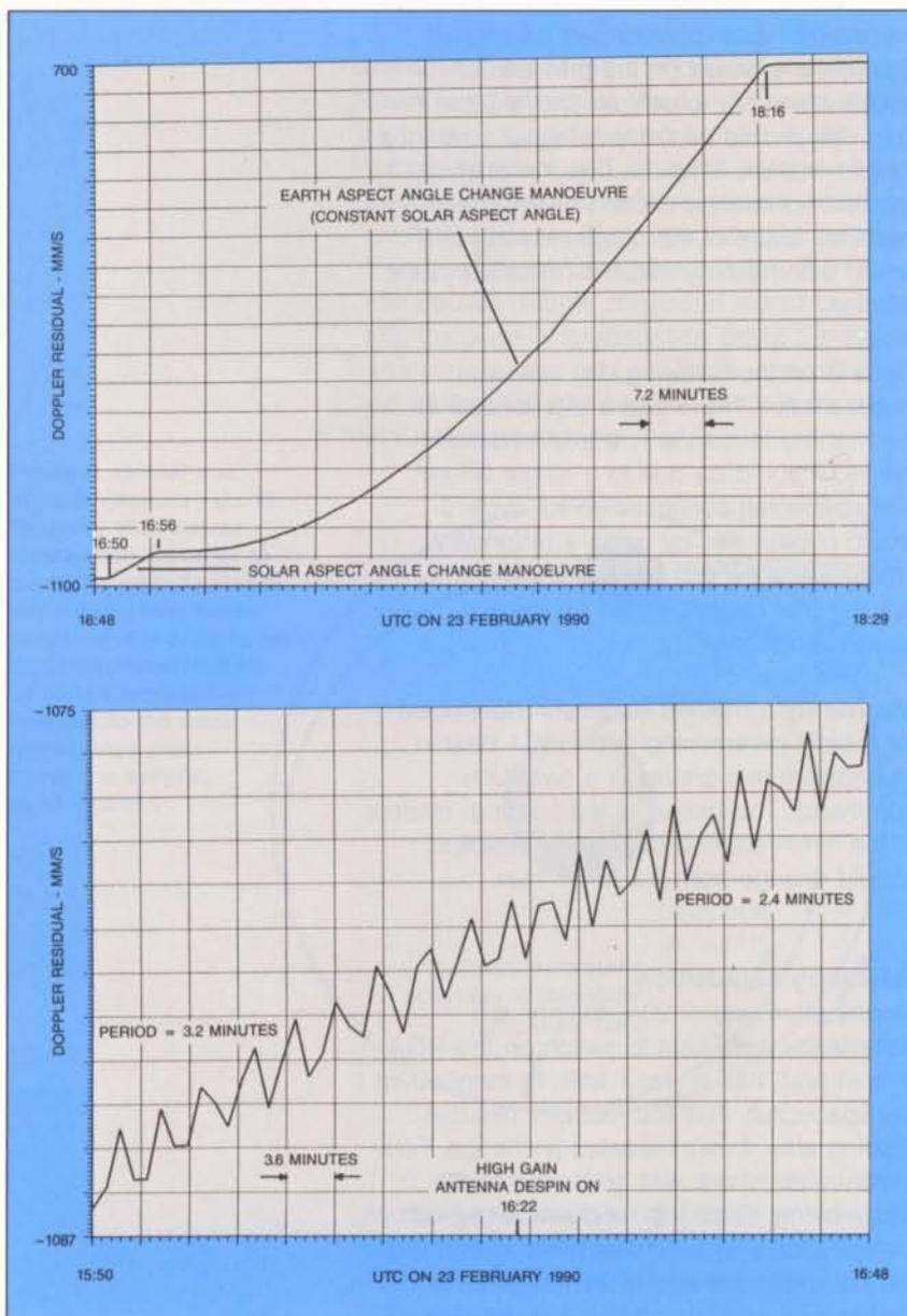
**Figure 6a.** The first reactivation manoeuvre as seen from the residuals of the 60 s count-time Doppler data obtained at the Madrid DSN station
