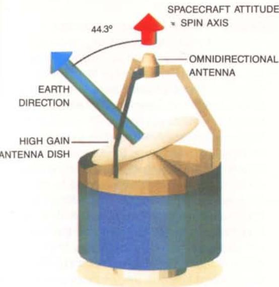
Figure 1. Schematic of the Giotto spacecraft showing the omni-directional Low-Gain Antenna (LGA) and the despun High-Gain Antenna (HGA)
