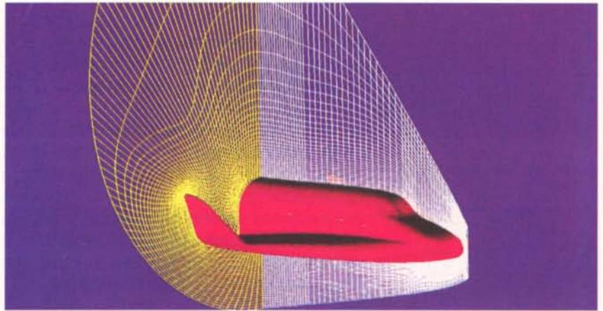
Figure 12. A typical structured volume grid for the Hermes spaceplane
