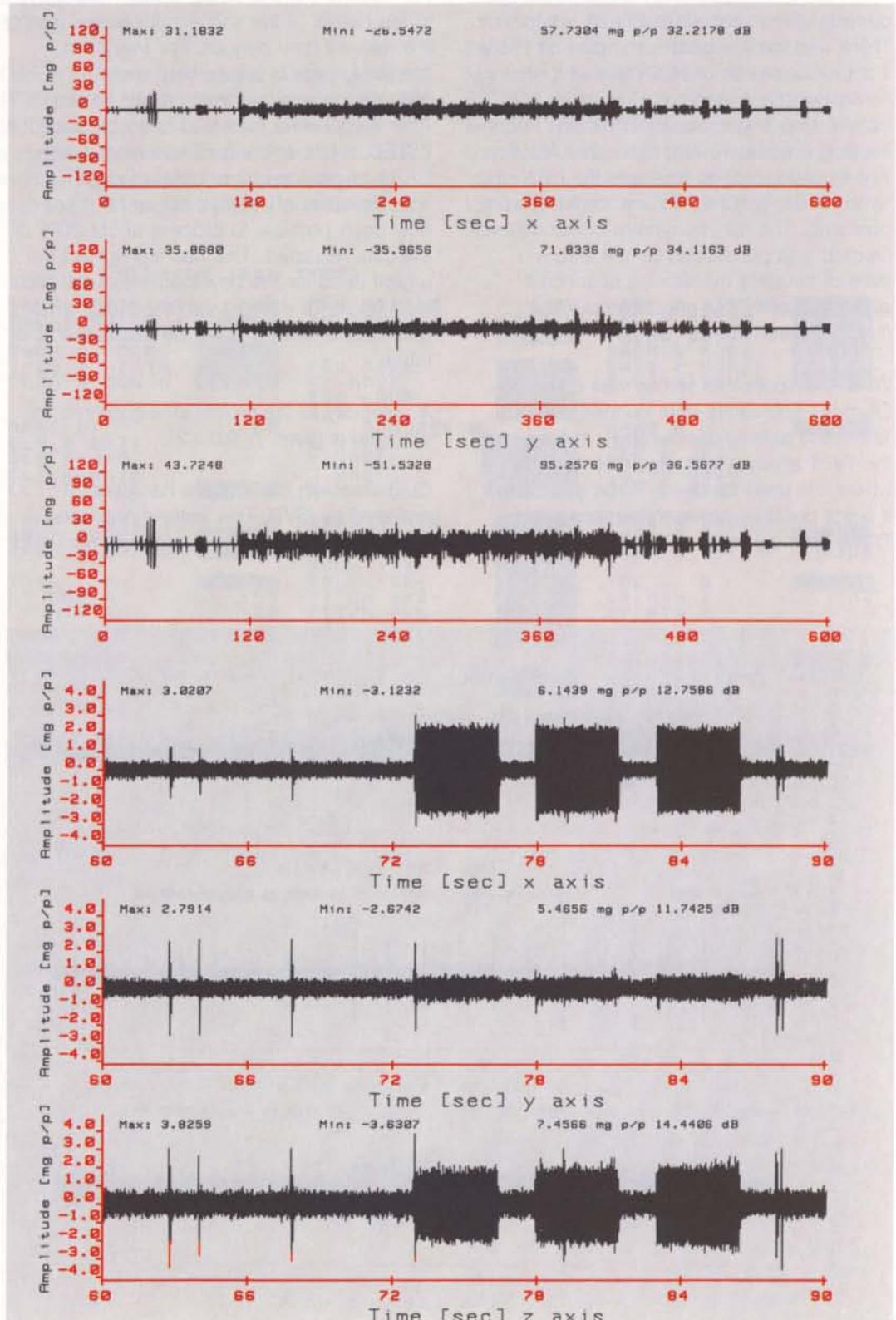
Figure 8b. 30s timeline plot showing normal stepping of one APM axis with blocks of 511 steps repeated at 5 s intervals, the first occurring after 73 s
