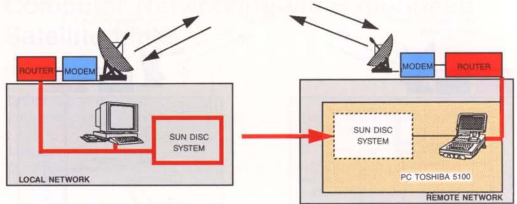
Figure 3. The setup for the publishing-package transmission test
