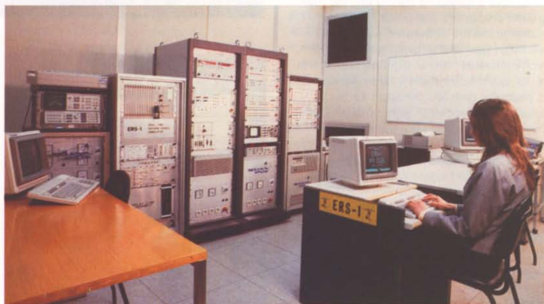
Figure 3. ERS Radar-Altimeter Electrical Ground-Support Equipment (EGSE) during its acceptance testing, at Selenia Spazio (I)
