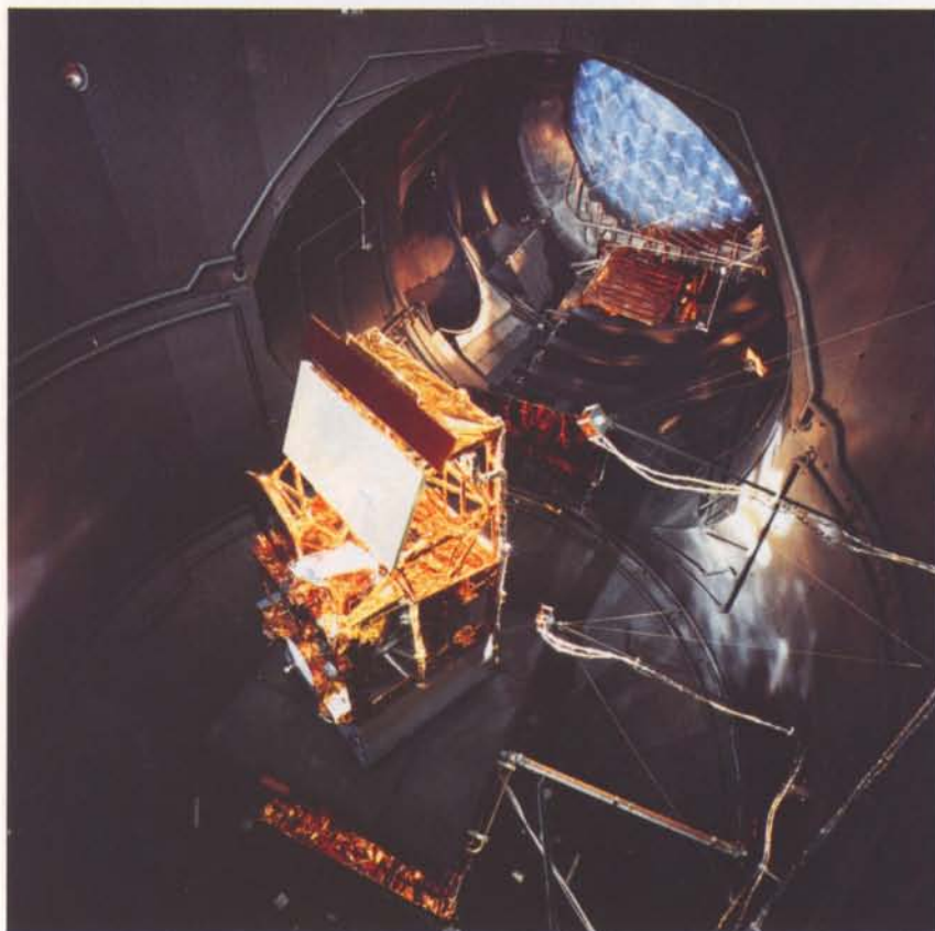
Figure 22. The ERS-1 payload during thermal-balance/thermal-vacuum testing. The antennas were fitted with heaters to simulate Earth-emitted radiation
