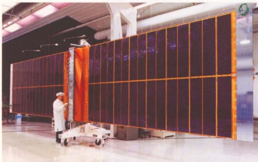
Figure 4a. Front side of the ERS-1 solar array (Photo. Aerospatiale)
