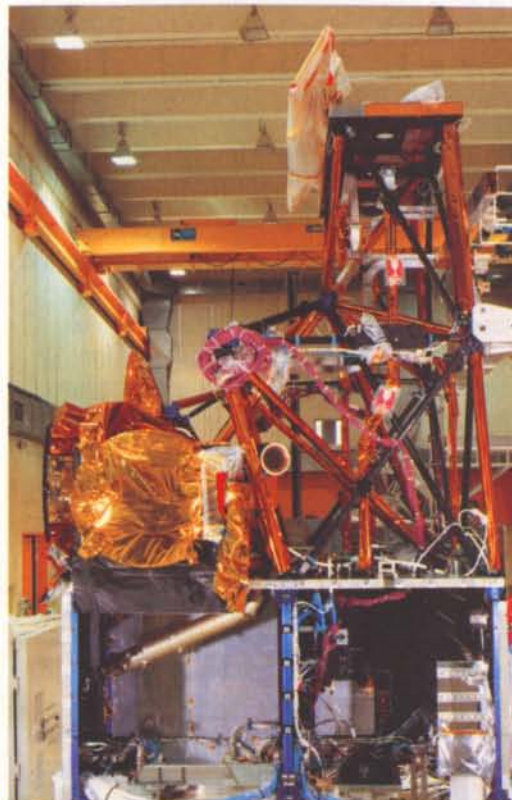
Figure 5a. The ERS-1 payload support structure, showing the box-like Payload Electronics Module (PEM) structure and the complex strut assembly of the Antenna Support Structure (ASS)
