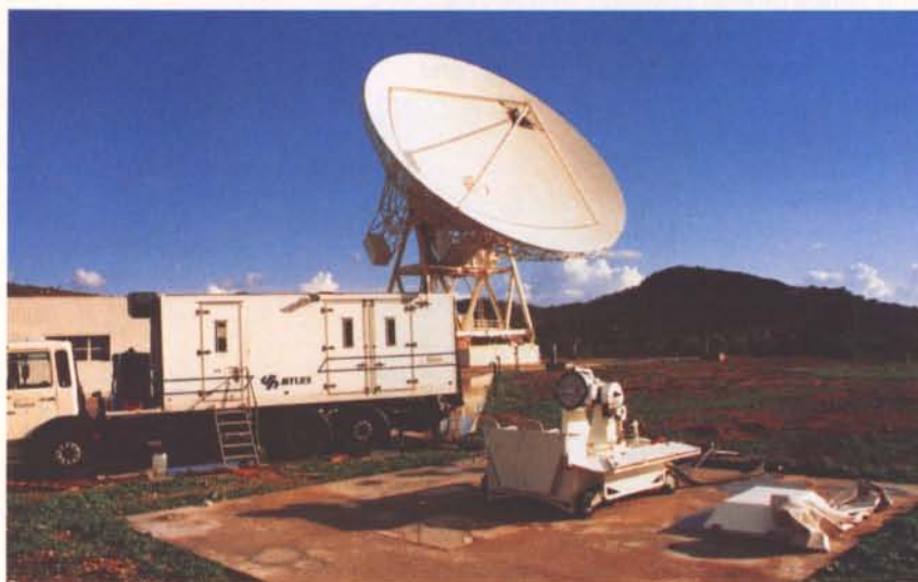
Figure 6. The mobile laser-ranging station, MTLRS-2, in Sicily in December 1990, from where it was transferred to the Venice site
