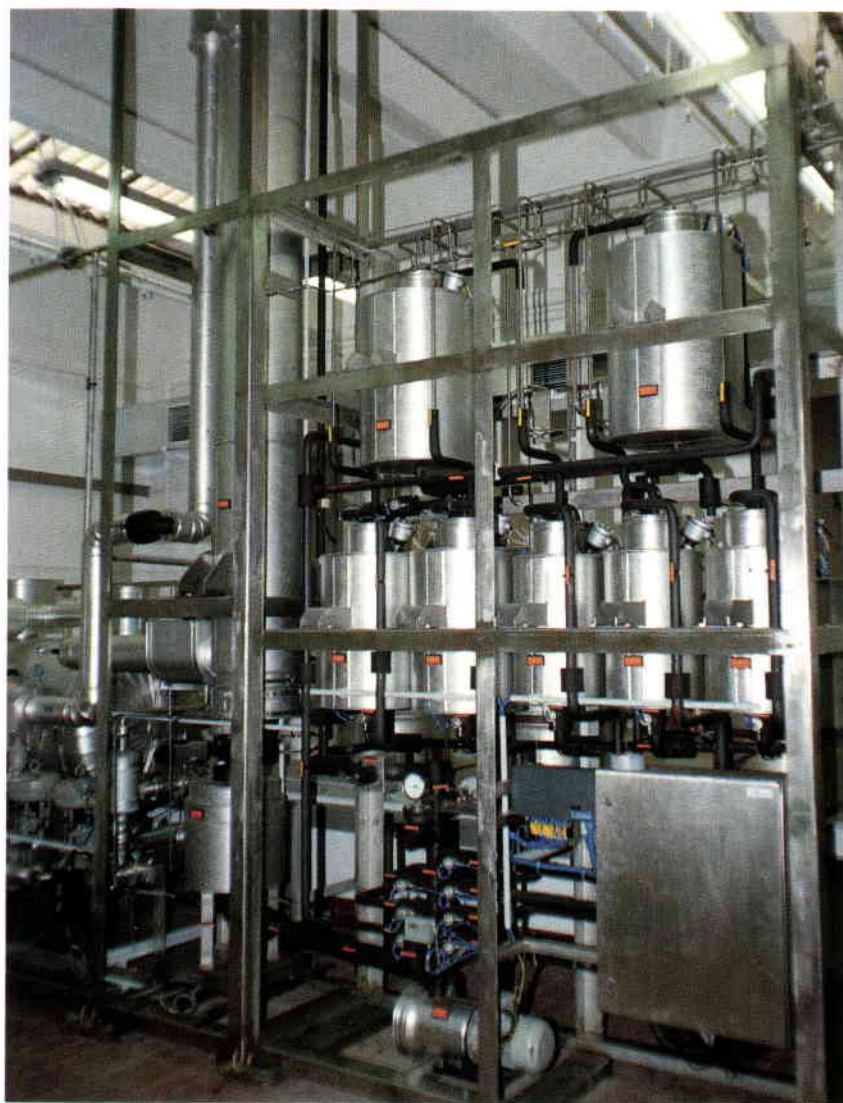
Figure 10. Hydrazine purification plant. To the left is the crystalliser and to the right the five stage vessels
