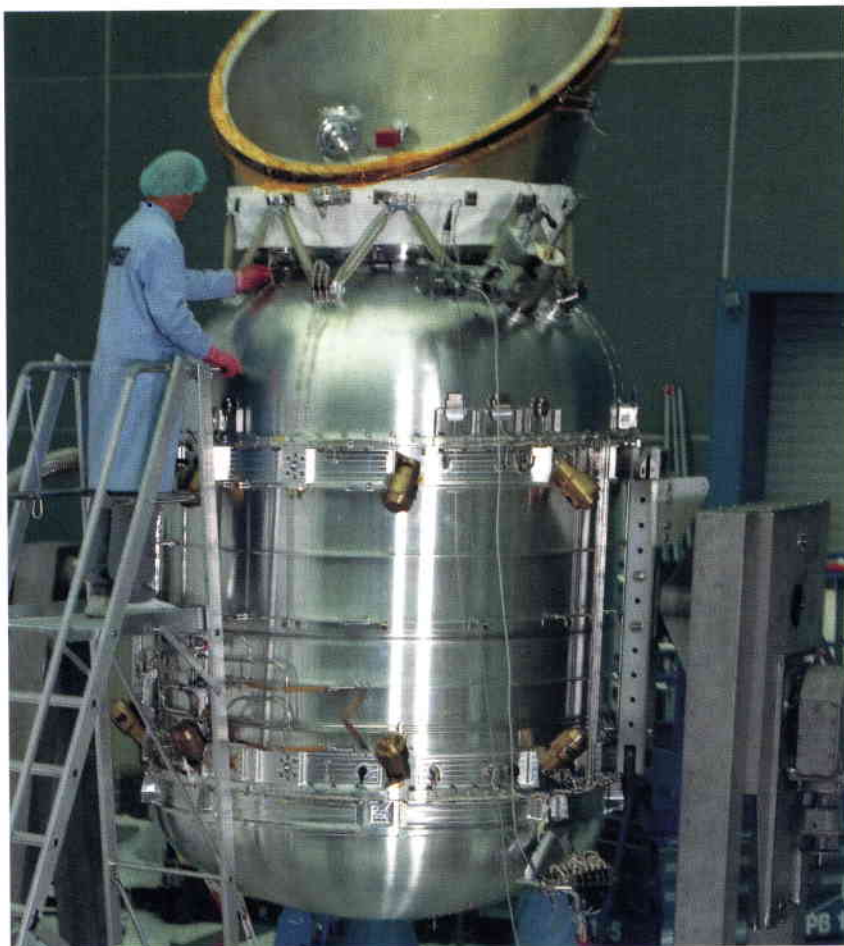
Figure 6. ISO Payload Module under test at MBB, Munich.
