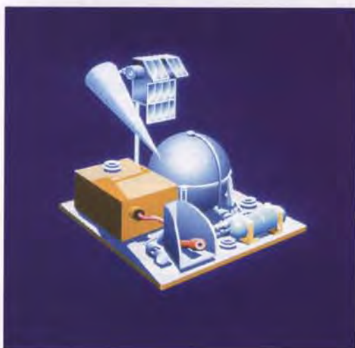
Figure 11. The Italian-developed low-power arcjet proposed for a flight test on Eureka-3, (the Diva experiment)
