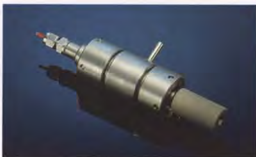
Figure 10. The two low-power arcjet thrusters being investigated at BPD and Centrosazio, in Italy
