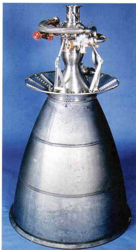
Ariane-5 upper stage (L9) AESTUS engine nozzle
