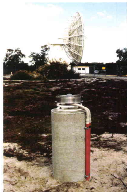
Figure 7. A GPS installation in Perth, Australia. The small GPS antenna (in the foreground) is mounted on a concrete pillar to achieve millimetre-level stability
