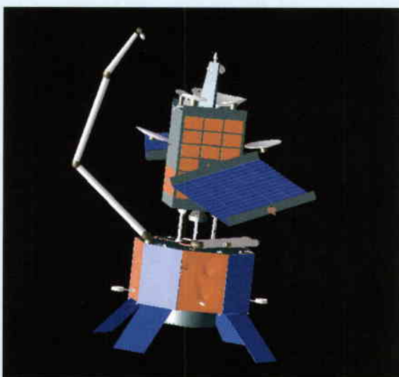
4f. One arm, with a camera on its tip, provides ground control with close-up images of the repair zone
