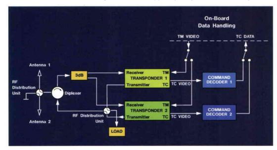
Figure 1. Architecture of a typical satellite TTC system
