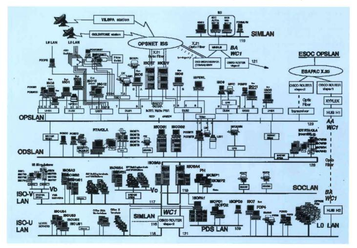
Figure 2. The ISO computers and Local Area Networks (LANs) at Villafranca operational issues. The final ITT System Operation Validation tests and operational simulations provided early feedback on both operational aspects and system performance. In addition, they offered an opportunity for the extensive training of operational personnel and ensured a smooth transition between the validation testing and the ISO pre-launch simulation campaign at Villafranca.
