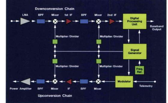
Figure 2. Block diagram of a typical TTC transponder. It comprises:
