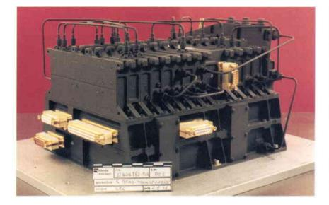
Figure 3. Standard S-band transponders (Photos: Alenia Spazio and Alcatel Espacio) In addition, the Doppler effects (frequency shift and frequency rate of change) when the satellite approaches perigee can be extremely high, which constitutes a further constraint for the receiver which must track these frequency dynamics.
