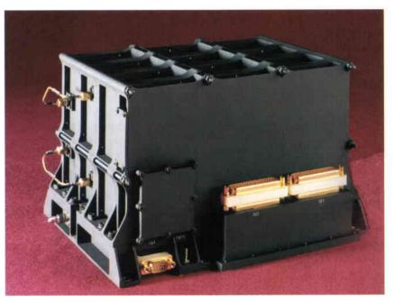
Figure 7. An Experimental S-Band Transponder (ESBT) (Photo: Alcatel Espace)
