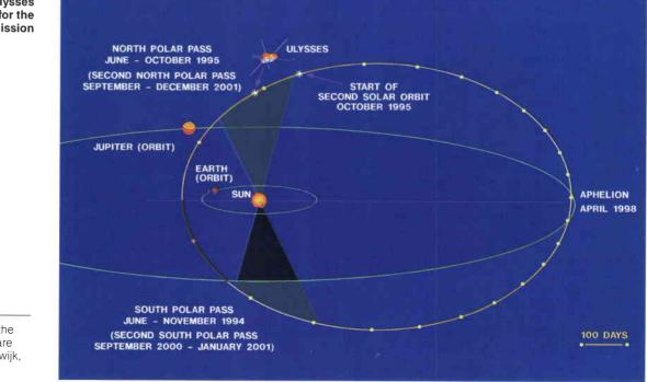
Figure 1. The Ulysses trajectory for the prime mission
