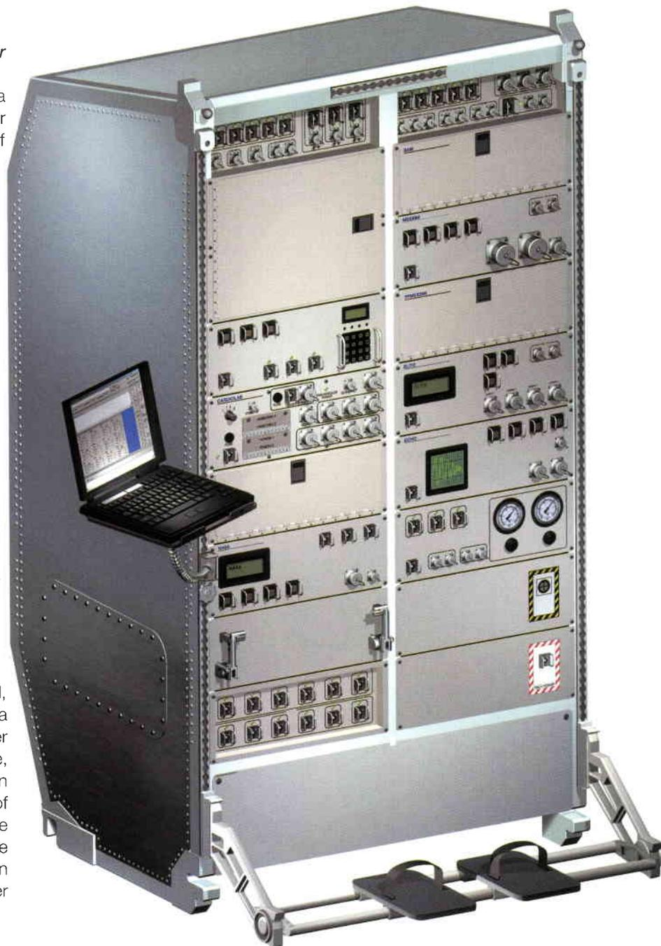
The SMs are accommodated in standard drawers of sizes of 4 PU and 8 PU (1 PU = 4.45 cm). They interface with the rack via a standardised guide system that simplifies the on-orbit exchange and installation of new SMs. All rack-mounted SMs are cooled via a ducted air system provided as part of the Carrier.
