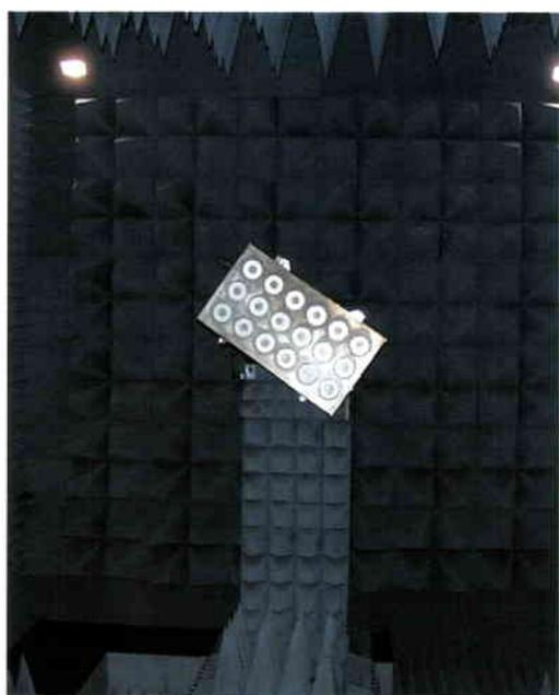
Figure 7. Anechoic chamber testing of the GRAS antenna breadboard developed within the EOOP and GSTP programmes (courtesy of Saab Ericsson Space)
