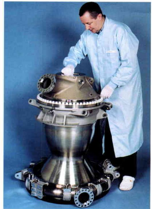
The Vulcain-2 nozzle extension was delivered in March 1999 for the engine test campaign, following delivery the chamber in the previous November. Preliminary assembly of the Vulcain-2 engine had also begun in November 1998, and it was delivered on 7 April 1999 to the P5 test rig in Lampoldshausen (D), operated by the German Aerospace Centre (DLR). The second PF50 test rig in Vernon (F), operated by SNECMA, received the second engine at the beginning of October 1999.
