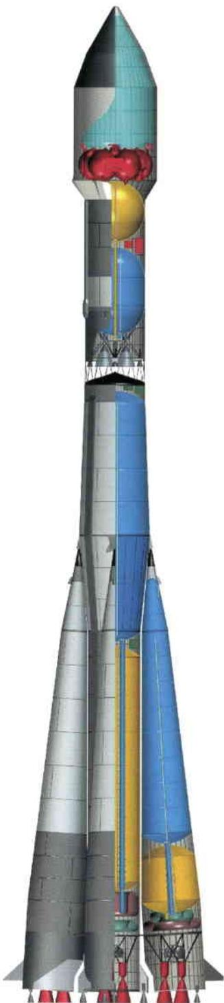
Figure 7. Cutaway view of Soyuz-Fregat
