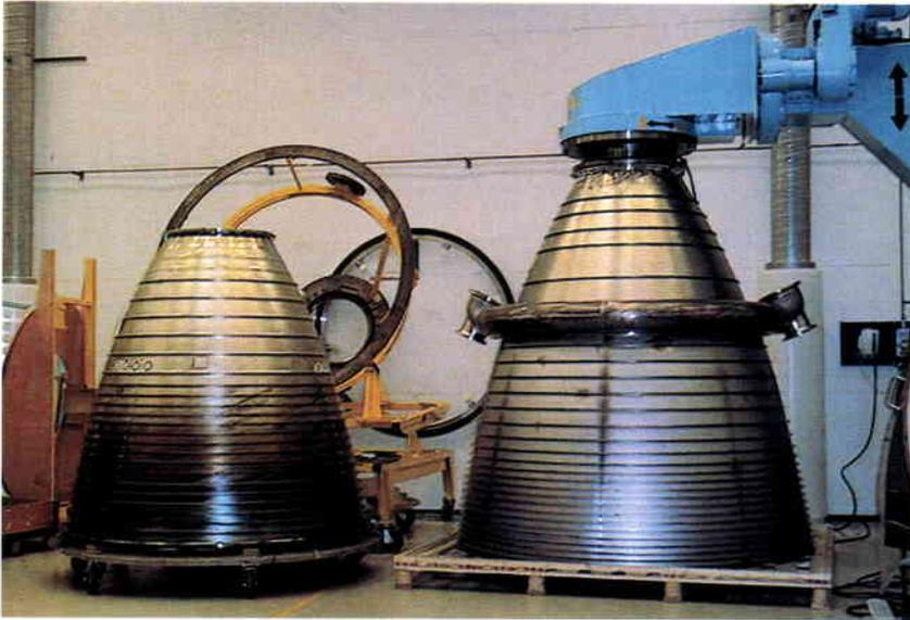
Figure 3. Vulcain and Vulcain-2 nozzle extensions
