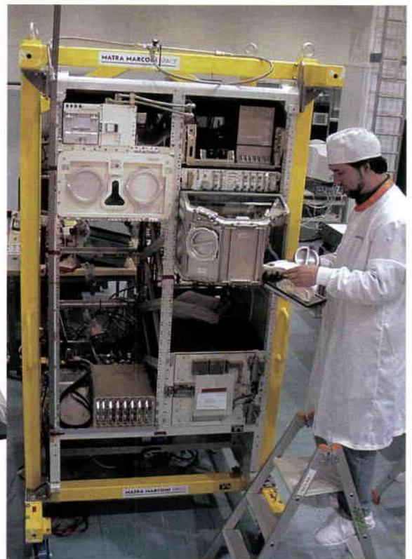
Figure 5. The Biolab Engineering Model under integration. (ESA/MMS-F)
