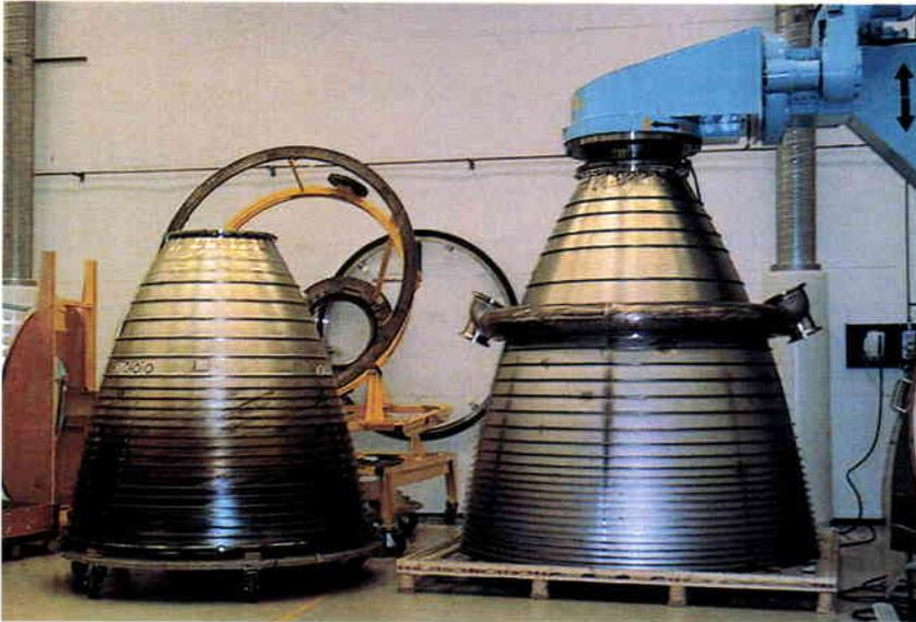
Figure 3. Vulcain and Vulcain-2 nozzle extensions
