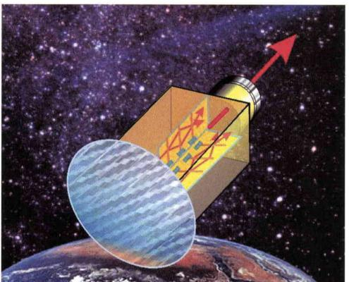
In a Mach-Zehnder interferometer, slowly drifting atoms are coherently split, re-directed and re-combined such that the atomic trajectories enclose as large a surface as possible. Beam splitting is achieved by atom-light interaction. During each interaction sequence, the atoms cross two counterpropagating laser beams. An atom absorbs a photon from one laser beam and is stimulated by the other laser beam to re-emit the photon.
