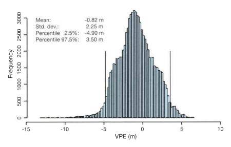
Figure 7. Typical ESTB vertical-error histogram
