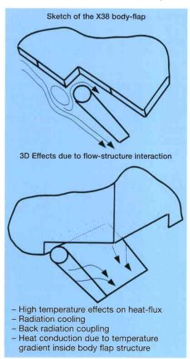
Figure 6. Sketch of complex flow-structure interaction on the X-38 body flap
