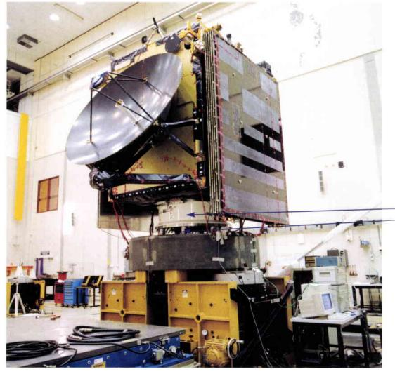
Figure 4. Rosetta STM mounted on the Force Measurement Device (FMD)
