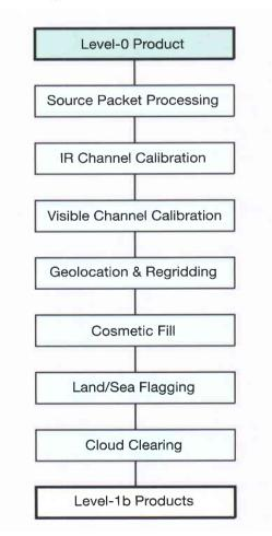
Figure 8. The AATSR Level-1b processing steps
