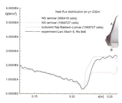
Figure 5. Predicted laminar and turbulent heat-flux distribution along the X-38's deflected body flap and a comparison with NASA LARC Mach 6 experiments
