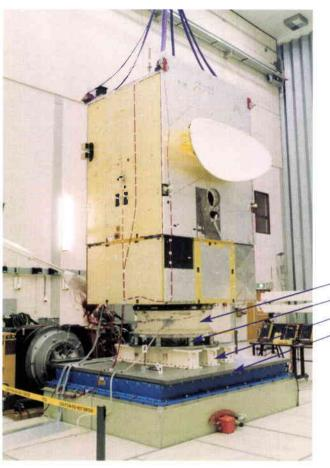
Figure 3. The Olympus STM mounted on the Force Measurement Device (FMD)
