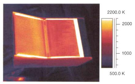
Figure 7. Surface-temperature distributions in the TETRA X-38 body-flap model with closed and open gaps in the L3K facility at DLR in Cologne
