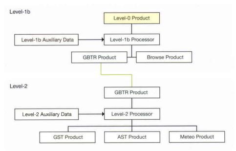
Figure 7. Relationship between the AATSR products and processing levels
