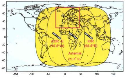
Figure 5. Inmarsat and Artemis EGNOS geostationary-satellite broadcast areas
