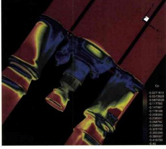
Figure 11. Surface mesh and preliminary predicted pressure distributions around an Ariane-5 model in NLR's HST facility for Mach 0.7 conditions
