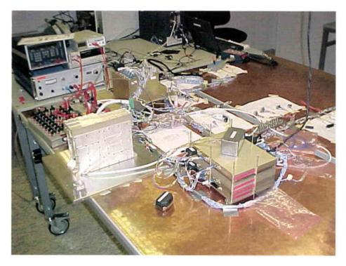
The three Smart-1 main avionics unit electrical models – the S-band Transponder, the Power Control and Distribution Unit, and the System Unit (left to right in the centre of the photograph) – being tested in the Bench Test Model set-up at the Swedish Space Corporation's premises in Solna
