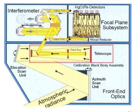
elevation scan unit controls the LOS viewing direction according to pre-defined tangent altitudes, and also the pointing to high altitudes (~200 km) required for radiometric offset correction ('deep-space' calibration).
