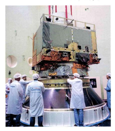
The SM includes eight batteries, and the solar array. This is a flat-pack array designed for the Polar Platform by Fokker Space (NL), based on their standard design elements. Once deployed, the array is rotated to point continuously towards the Sun using a solar-array drive mechanism, which is attached to the base of the central cone.
