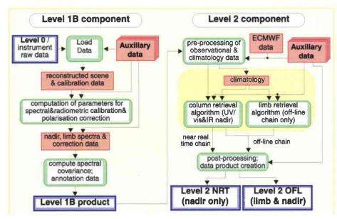
Figure 14. The SCIAMACHY ground-processing chain
