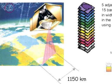
5 adjacent identical cameras 15 bands programmable, in width and position, in the range 390 to 1040 nm, using a CCD array.
