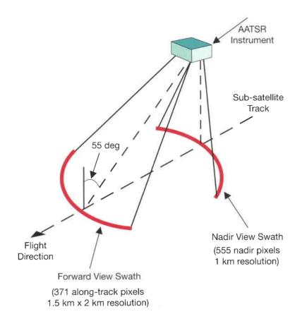
Figure 4. The AATSR viewing geometry (courtesy of RAL) procured by the UK Department of the Environment, Transport and the Regions (DETR), in partnership with the Australian Department of Industry, Science and Resources (DISR) and the UK Natural Environment Research Council (NERC).
