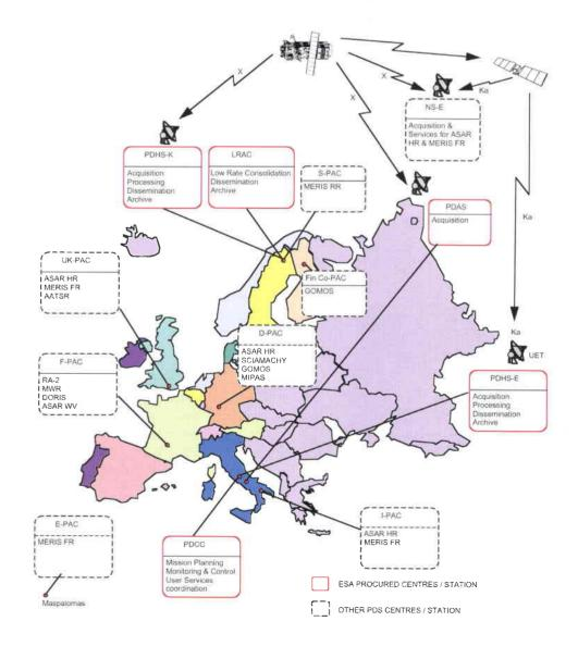
Figure 1. Locations and primary functions of the various Payload Data Segment (PDS) centres and stations
