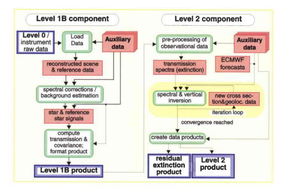
Figure 6. The GOMOS ground-processing chain
