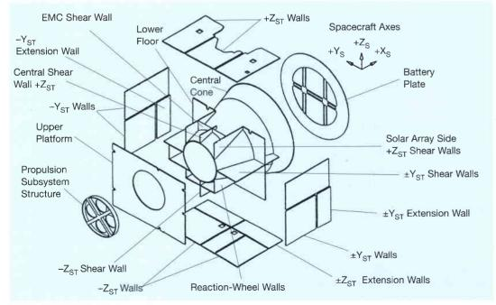
Module box structure around the central tube
