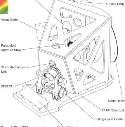
Figure 3. The ATSR instrument
