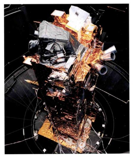
Figure 12. The complete Envisat payload in the LSS at ESTEC
