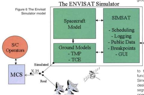
The Simulator runs on a DEC-Alpha work station and uses a generic 1750 emulator to model the satellite's on-board Central Communications Unit (CCU) and Payload Module Computer (PMC). This means that the actual flight software for both the CCU and the PMC can be executed in the Simulator, vastly adding to the realism and validity of the simulation.
