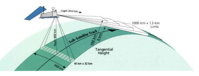
Figure 11. The SCIAMACHY viewing geometry
