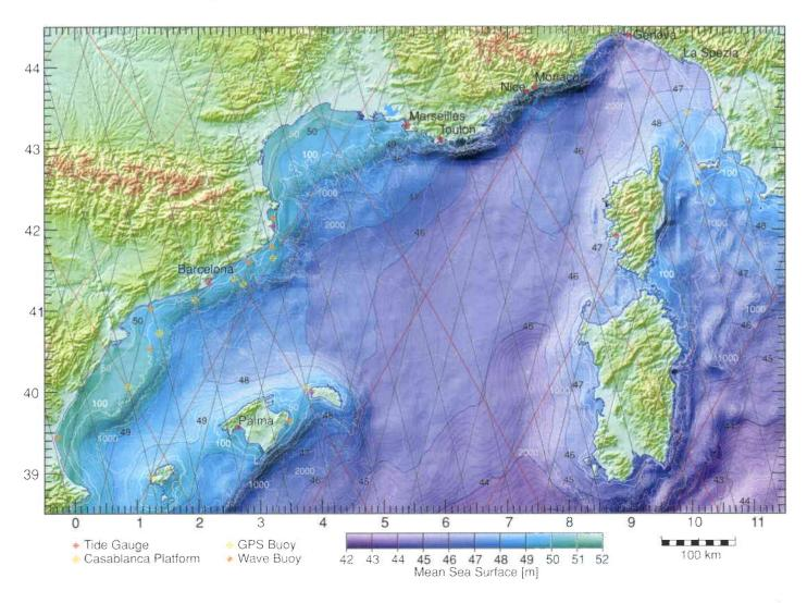
Figure 10. The northwestern Mediterranean Basin used as reference surface for the Radar Altimeter absolute range calibration (the Envisat ground tracks are shown) wave height and sigma-0/wind.
