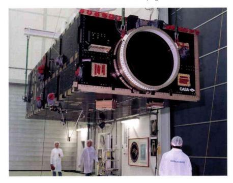
Envisat's size made it impractical to design a container to fit the integrated satellite into the AN124, which is largest commercially available cargo aircraft. Consequently, the Service Module, Payload Module, ASAR antenna and solar array will be transported separately and the satellite reassembled in Kourou.
