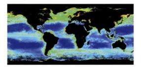
ATSR instruments flown on ERS-1 and 2, thereby ensuring the production of a nearcontinuous, 15-year dataset of Sea-Surface Temperatures (SSTs) at an unprecedented accuracy level of 0.3 K or better (Fig. 2).
