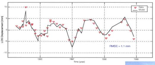
Figure 14. Measured line-ofsight displacement of the La Vilette Science Museum in Paris, compared to the modelled displacement due to temperature variations (courtesy of Politecnico di Milano, I)
