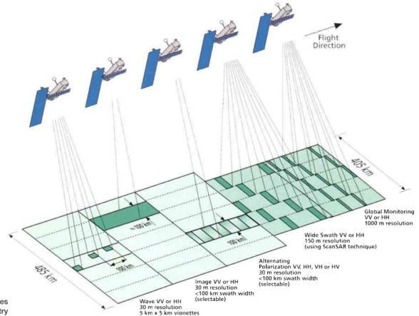
Figure 4. The ASAR modes and observation geometry
