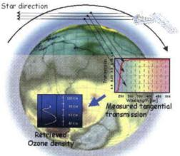
Figure 3. GOMOS viewing geometry and measurement principle. The left panel illustrates the instrumentpointing envelope (range of all possible pointing directions), whilst the right panel shows an occultation sequence. As the satellite moves away from the star, it will appear to fall behind the horizon. As the atmosphere occults the star, the acquired spectra will increasingly show absorption features (due to ozone and other gases)
