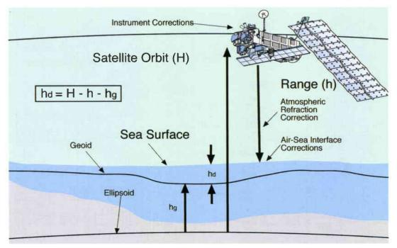
Figure 12. RA-2 derived height measurements
