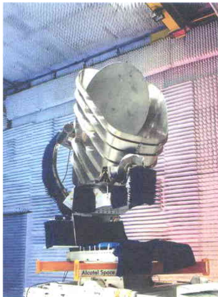
RF testing of a Planck development model
