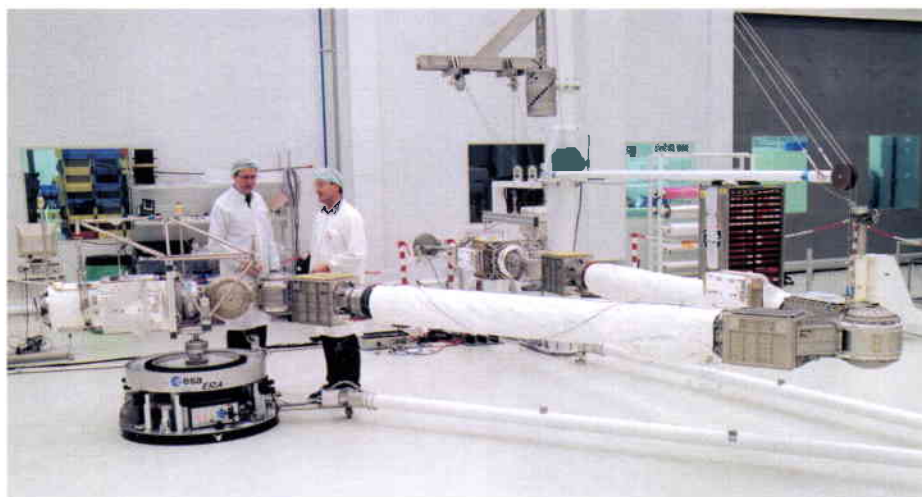
ERA Robotic Arm flight model at Fokker Space
