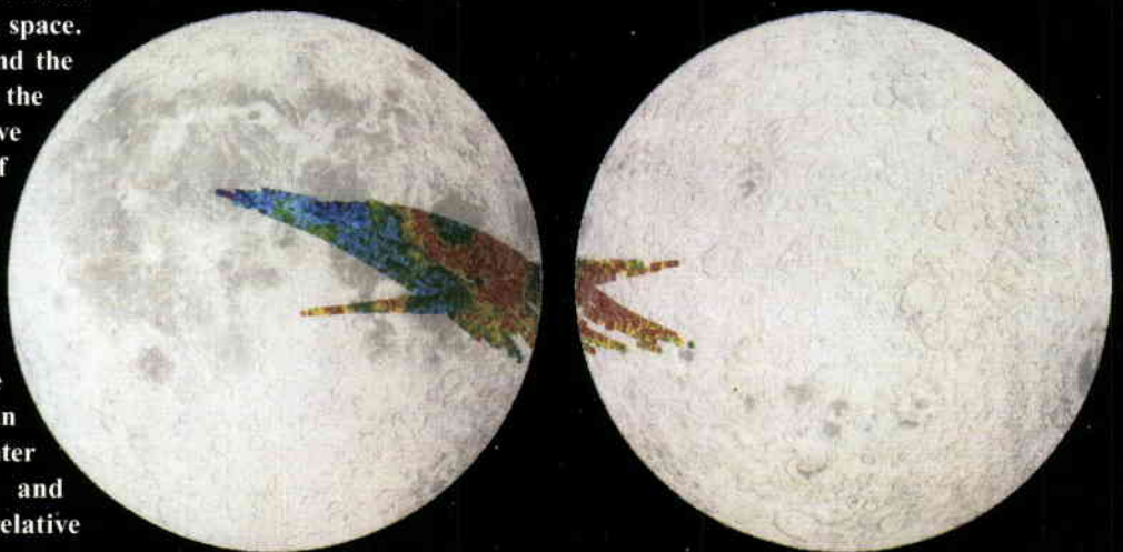
Compared to Apollo silicon/aluminium ratio maps over 10% of lunar surface, D-CIXS will have global X-ray cover and will determine absolute chemical element abundances.
