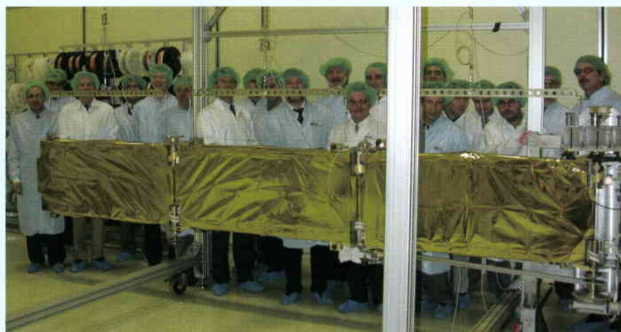
Three-segment arm deployment testing of the MIRAS Demonstrator for SMOS
