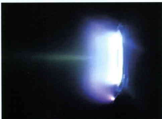
The SMART-1 electric-propulsion thruster firing in the ESTEC test chamber. The plume is visible due to the excited xenon (Xe+) ions: the central part shows a greenish light (high-energy emission), while the ions close to the cathode, on the right, emit a reddish glow (lower energy). The white annular core is where the plasma (Xe+ and e-) is generated, maintained and accelerated
