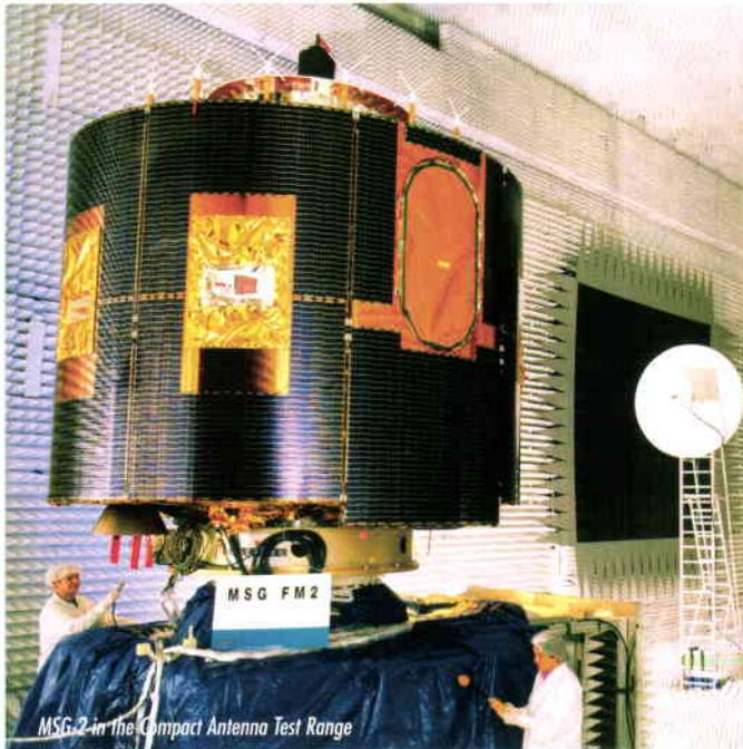
MSG-2 in the Compact Antenna Test Range
