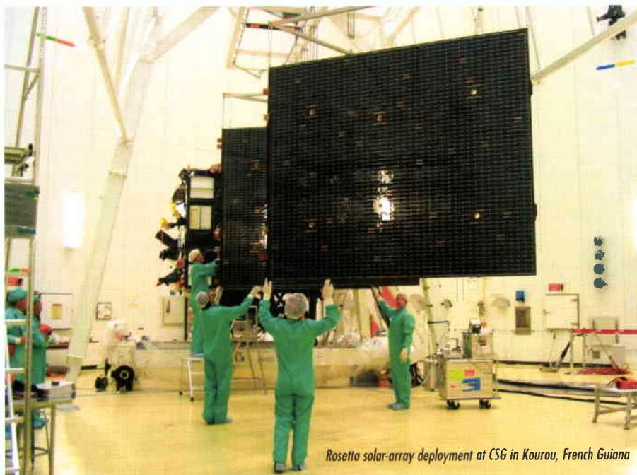
*Rosetta solar-array deployment at CSG in Kourou, French Guiana*
