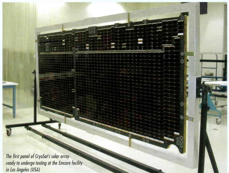
*The first panel of CryoSat's solar array ready to undergo testing at the Emcore facility in Los Angeles (USA)*
