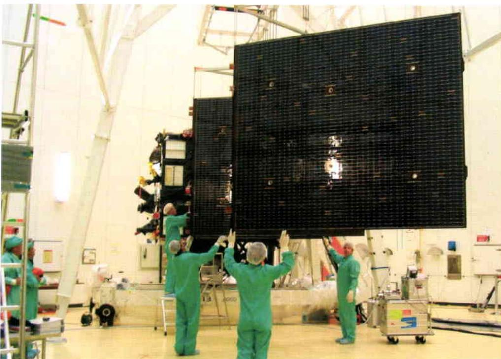
*Remounting of the solar arrays in Kourou*
