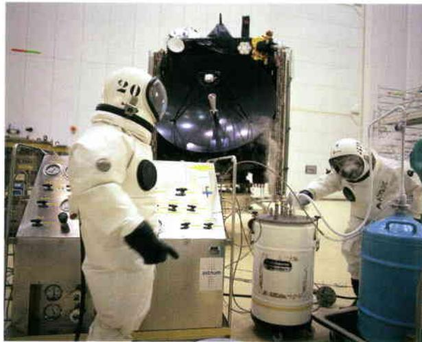
*Fuel being offloaded from the Rosetta Orbiter after the first launch's postponement*
