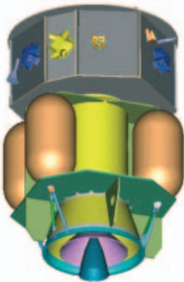
*CAD drawing of the LISA Pathfinder spacecraft, with the science package containing the LTP and the DRS sitting atop the propulsion module, which will carry it out to the L1 halo orbit*
