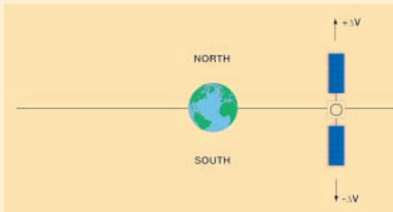
*The geostationary orbit and the concept of tangential and out-of-plane burns*
