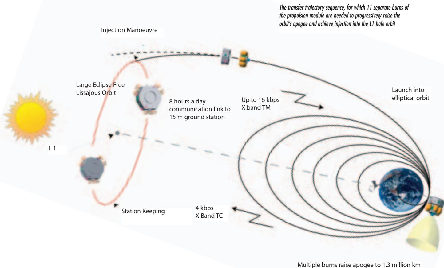
environment in terms of 'tidal forces' (produced in the vicinity of massive bodies, from which L1 is sufficiently far away), thermal stability, magnetic field, and radiation, is reachable year-round, and also allows daily visibility from a single ground station. The 'halo' in fact is a three-dimensional orbit with a shape similar to the contour of a potato chip.
