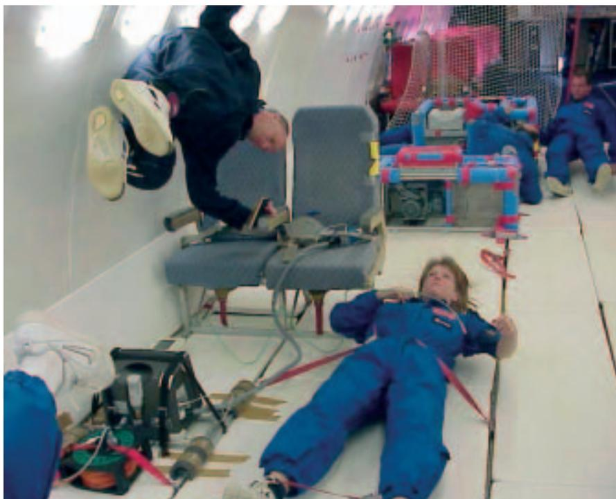
*Dr P. Norsk monitors Dr B. Pump acting as the test subject for the measurement of arterial blood pressure during the 25<sup>th</sup> ESA Parabolic-Flight Campaign in October 1998*
