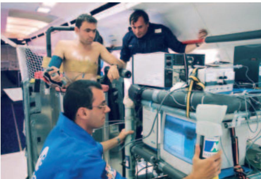
*A test subject standing in the LBNP caisson while his heart rate and blood pressure are monitored for the experiment of Prof. P. Vaida during the 30<sup>th</sup> ESA Parabolic-Flight Campaign in May 2001*
