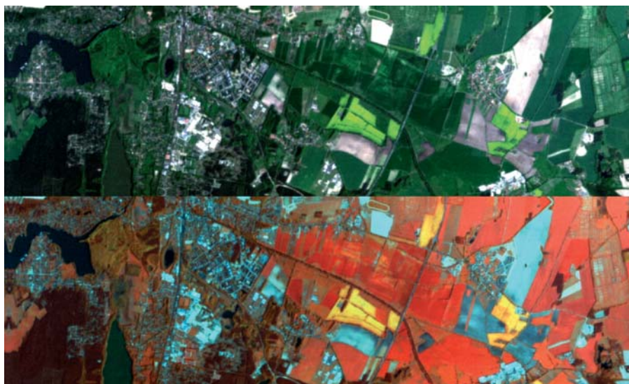
Simulated Sentinel-2 colour composite images using the red/green/blue bands (above) and near-infrared/red/green (below)
