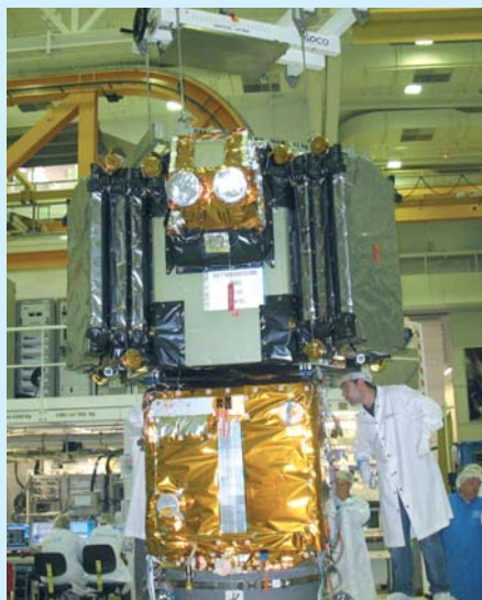
Left: the SMOS payload meets its Proteus platform in Cannes; the SMOS satellite is born!
