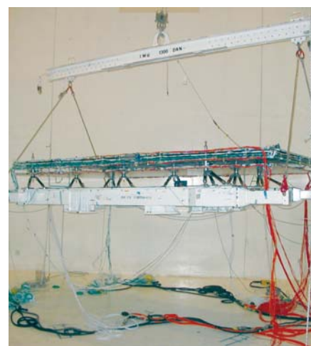
Preparing for the acoustic vibration test to simulate the rigours of launch
