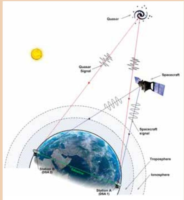
Delta-DOR tracking of a deep-space probe and of a nearby quasar from DSA-1 (New Norcia, Australia) and DSA-2 (Cebreros, Spain). The effects of common error sources between spacecraft and quasar observations are cancelled by the quasar tracking.
