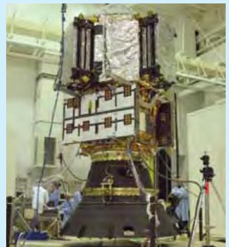
recorded pyrotechnic shocks were in line with the equipment qualification limits.
