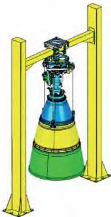
Expander Demonstrator mechanical test configuration (SNECMA Moteurs)
