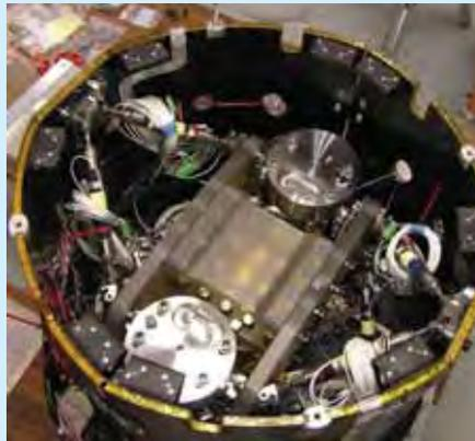
*The LISA Technology Package Central Assembly mounted inside the LISA Pathfinder science module flight structure under vibration test at Astrium GmbH in Friedrichshafen*
