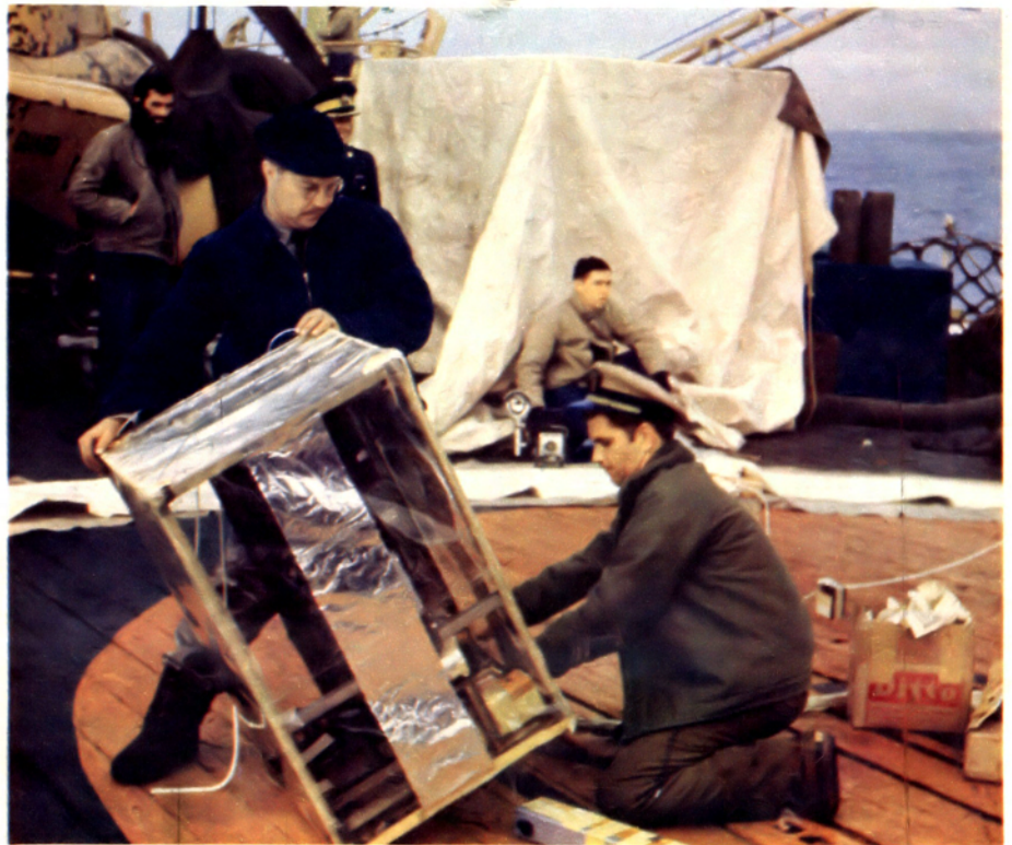
Left: high-altitude cosmic-ray tests were carried on from Coast Guard cutter Eastwind by launching balloons which set off rockets aloft. Above: preparing rocket-firing mechanism
