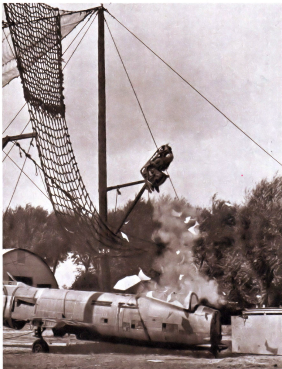
Ejection seat, similar in principle to escape capsule, being tested by Navy. Military services use ejection for bail-out from fast jet planes
