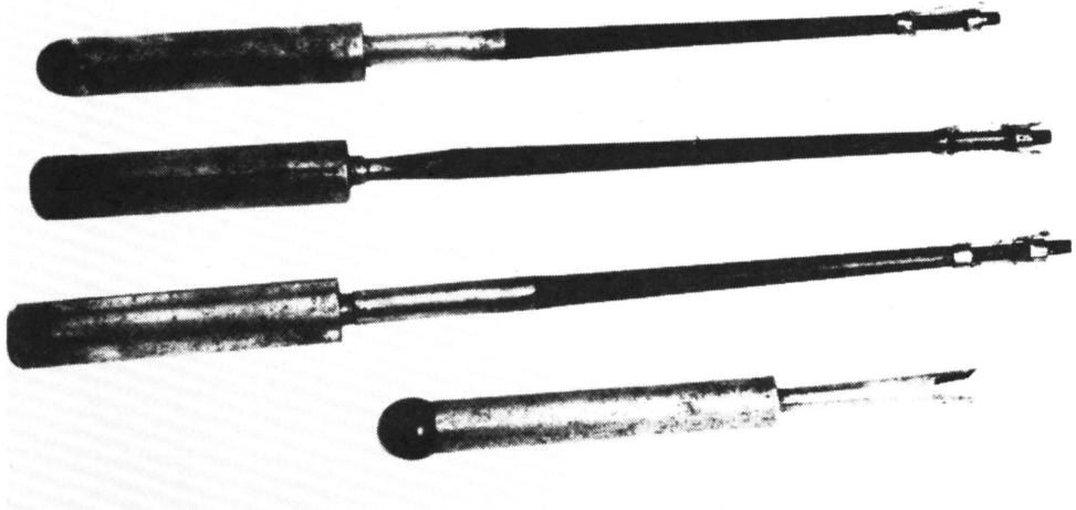
Figure 13 Three incendiary rockets with rotating fins - shell rocket. Congreve C. 1823 (Science Museum neg. 1476/85).
