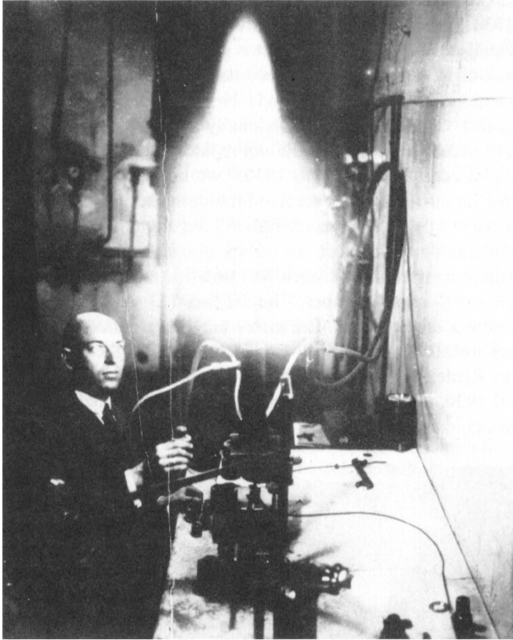
Figure 2 Max Valier (1895-1930) experimenting with a gaseous oxygen/alcohol rocket motor, probably at the Heylandt plant, March 1930. Imperial War Museum photo.
