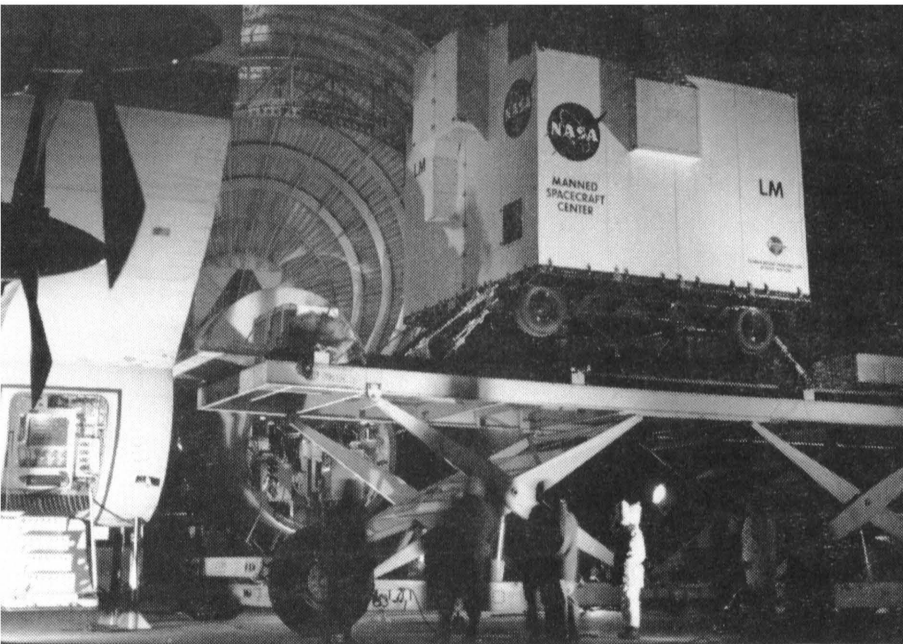
Figure 21 LM Ascent Stage in Sealed Shipping Container Being Loaded Aboard Super-Guppy Transport Aircraft.
