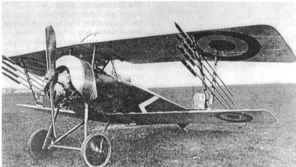
Nieuport 17 of 110 hp and 15 m 2 with 8 rockets.
