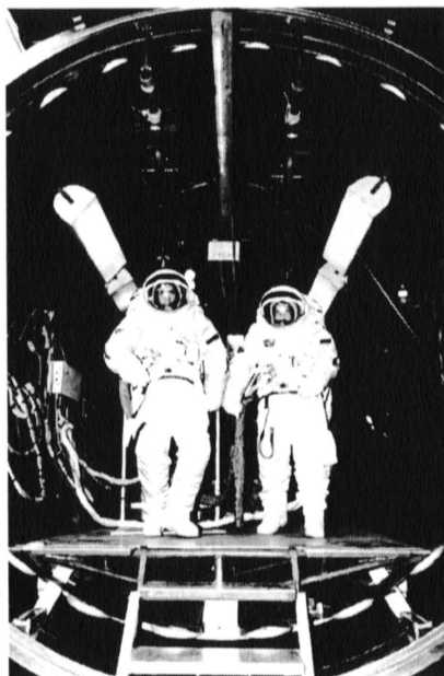
Figure 3: Orlan-type suit testing in the TBK-50 thermal and vacuum chamber at Zvezda. Credit: Archive Zvezda.
