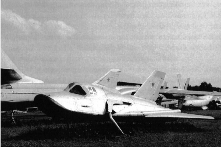
Figure 3–9: The EPOS, a manned “analogue” (demonstrator) of the OS, which was being used for in-atmospheric subsonic flights, in the Russian Air Force Museum. Credit: Photo by the author.
