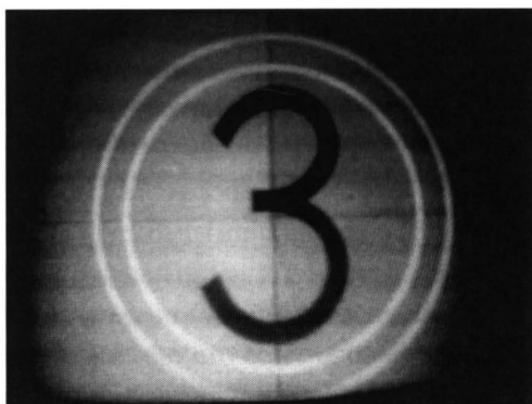
Figure 20–3: Horizontal lines are visible when the refresh rate of the projector and receiver are not fully in phase. These lines appear to move slowly down the screen.
