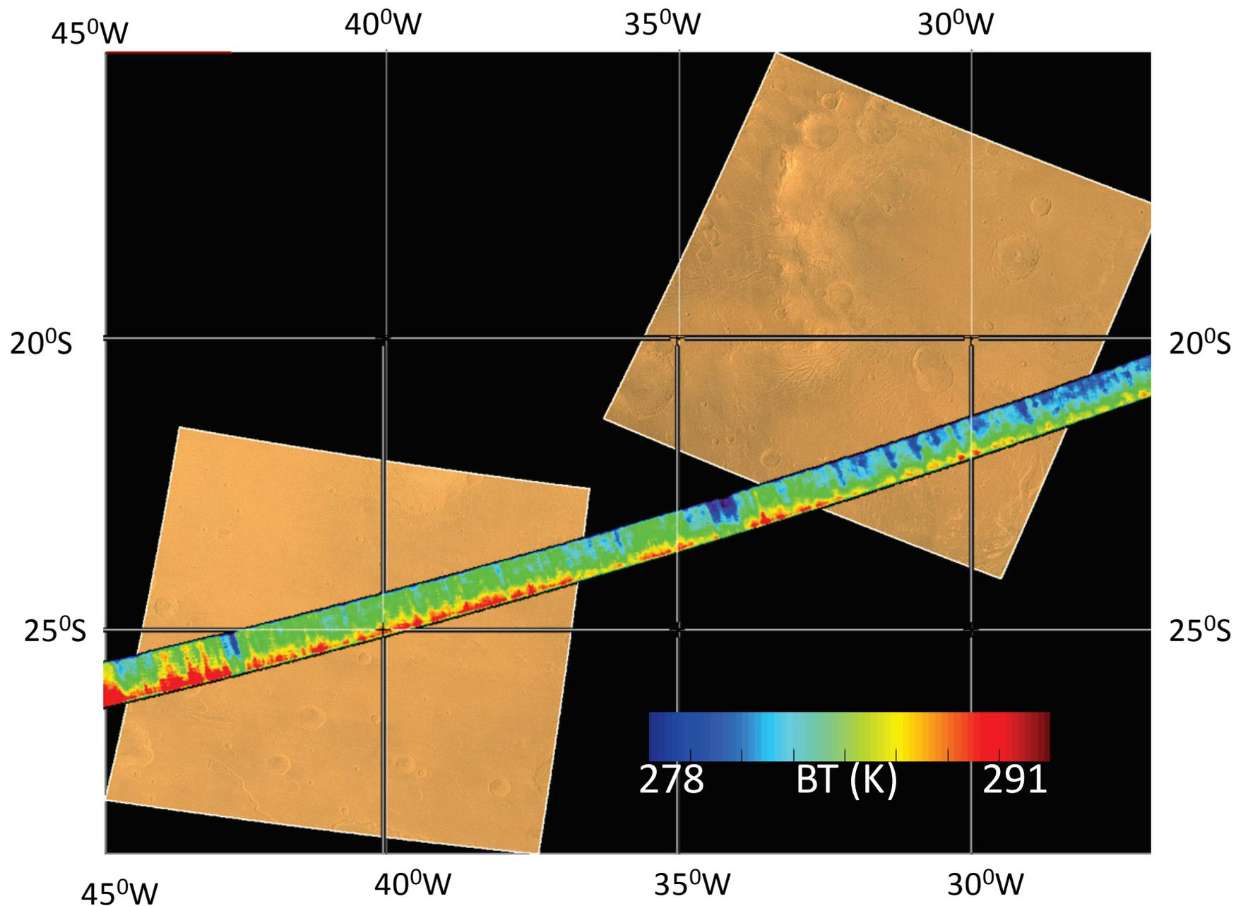
Brightness Temperature (BT) variability as observed from push broom imaging from TIS instrument near Holden Crater on 27 Feb. 2015 (Ls=299.2 Degrees) in 10.25  $\mu\text{m}$  spectral band from the altitude of 386 km. TIS observations are draped on background of MCC data as ancillary source of information.
