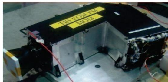
Thermal-Infrared Imaging Spectrometer
