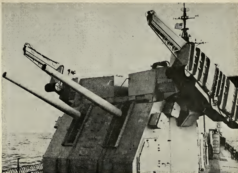
THE ROCKET-ASSIST TORPEDO (Rat) launching system utilizes the after five-inch gun mount and fire control system of destroyer to provide an anti-submarine weapon of greatly improved accuracy and extended range of about five miles. Solid propellant first stage by Allegheny Ballistics boosts torpedo into flight and propels it along ballistic flight path to general vicinity of submarine. Nose cone and parachute separate as Rat enters water to acoustically home on target.
