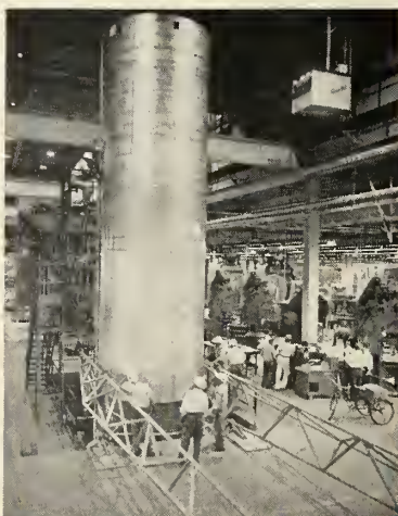
JUPITER AND REDSTONE ballistic missiles move down parallel production lines at the Warren Missile Plant of Chrysler. The number of Jupiters shown indicates quantity production is being achieved. A Jupiter tank assembly undergoes dynamic tests at the missile plant (right). The missile section has been lowered into a test pit below the floor level for this operation. Heavy presses and other production equipment used for manufacture of components can be seen in the background.
