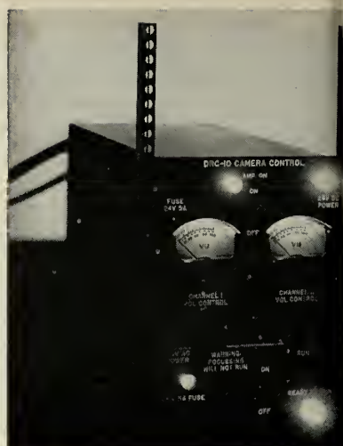
DRC-10 control unit for remote use. Color lights show operational mode.
