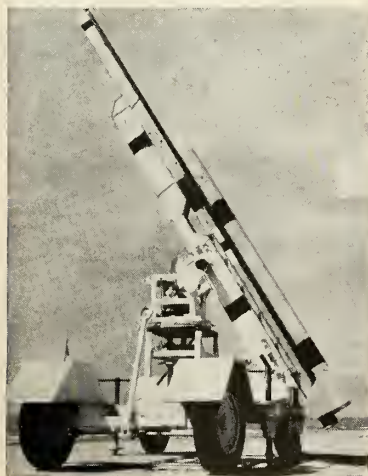
PHOTOGRAPHS AND DATA on the latest Japanese sounding rockets indicate a remarkable advancement in the state of the art. Both of the rockets shown were developed by Professor Hideo Itokawa, Institute of Industrial Science, University of Tokyo. Itokawa is head of Japanese IGY sounding rocket program. K-150 rocket (left). Single-stage, solid propellant sounding vehicle fired April 8, 1958. Diameter—150mm. (5 \frac{1}{2} in.); length—3.3m (10 \frac{3}{4} ft); weight—70kg (154 lbs). Kappa Type V two-stage rocket (right) fired April 29, 1958. First stage diameter—220mm (8 \frac{5}{8} in.). Second stage—K-150 rocket. Maximum velocity—about 1,000 m/sec (3300 ft/sec).
