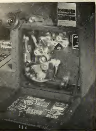
CAMERA with plug-in control unit for remote use showing magazine interior.
