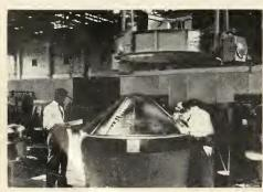
EVERY CONE arriving at the Cape receives a "pitplotting" inspection for possible shipping damage.
