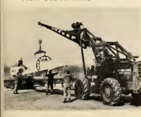
QUARTERMASTER Corps' "Ranger," all-purpose vehicle is being used to lift Nike-Hercules to its launching rack for union with the booster. It can pull 19,000 lbs. and lift 10,000 lbs.
