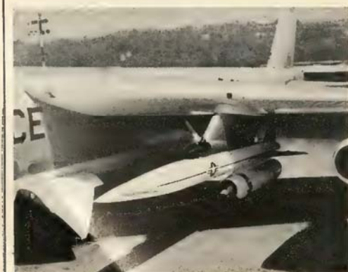
TRAINING and test model of North American GAM-77 Hound Dog rests on its pylon under wing of B-52. Test vehicle will have same aerodynamic characteristics as the operational bird.
