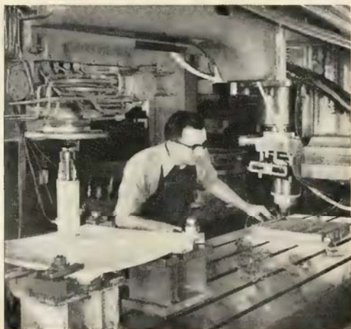
MARTIN has developed a "Hula Head" device where the cutter head performs a hip movement as it machines complex honeycomb parts. Modified stylus with five pick-up points converts a 3-axis cutter to a 5-axis.
