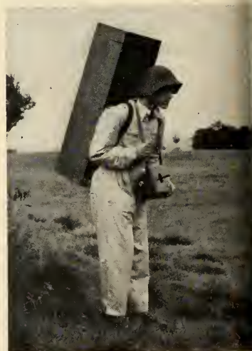
CONTAINER with two missiles weighs only 23 lbs. and is strapped on back
