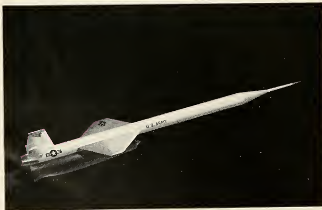
Ramjet-powered supersonic target, Lockheed Q-5 KINGFISHER electronically simulates enemy attackers—is being used by U. S. Army to evaluate and sharpen our nation's missile marksmanship, increase our defense capabilities.
