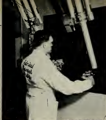
ADMIRAL CORP. nuclear engineer remotely handles components in the company's 20 kilonrie cobalt 60 radiation chamber.
