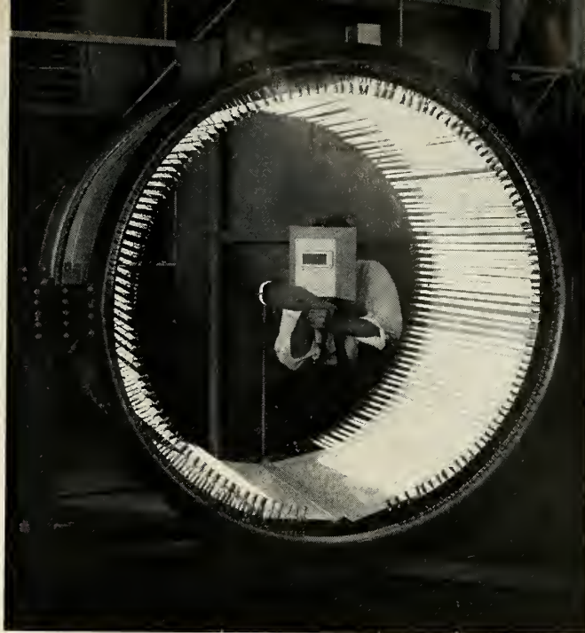
THIS OVEN —capable of testing components at 3000°F—is part of Convair's recently-opened High Temperature Structures Research Lab.
