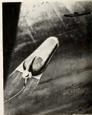
MARK 39 wire guided underwater missile may have 60-knot speed but in 1971 period torpedoes will require 200-300 knots.
