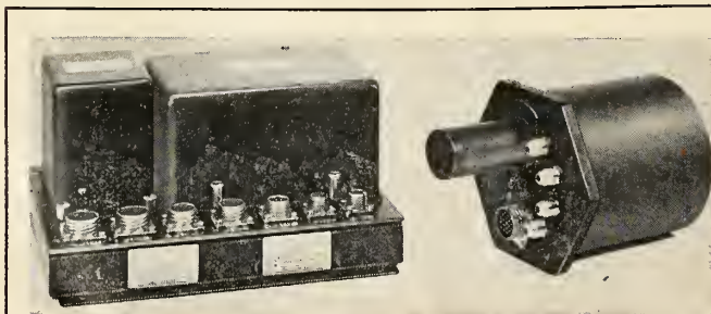
ABOVE: Servomechanisms' Type AQC 600 propellant utilization control system assures that the fuel and oxidizer are depleted simultaneously. This system measures the pressure ratio remaining in the tanks and controls flow. RIGHT: Schematic of the system.
