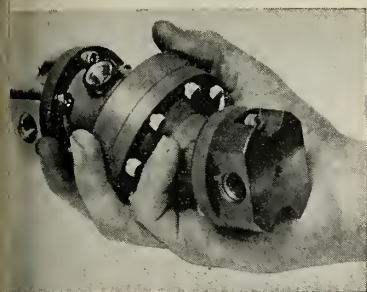
WICKERTS hot-gas motorpump. Unit shown, smallest in series, is capable of 1.9 hp and weighs only 2.5 pounds.
